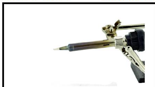
3. PROPERLY TINNED SOLDERING IRON TIP
