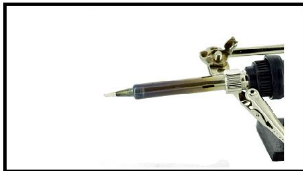
3. PROPERLY TINNED SOLDERING IRON TIP
