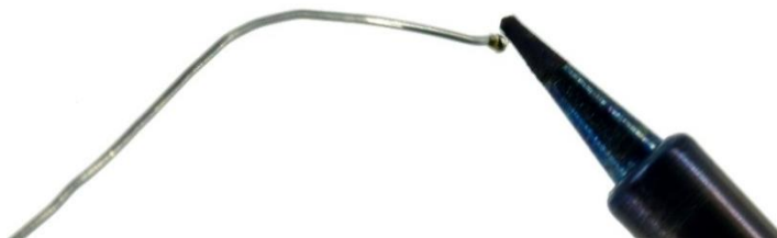
3. PROPERLY TINNED SOLDERING IRON TIP
