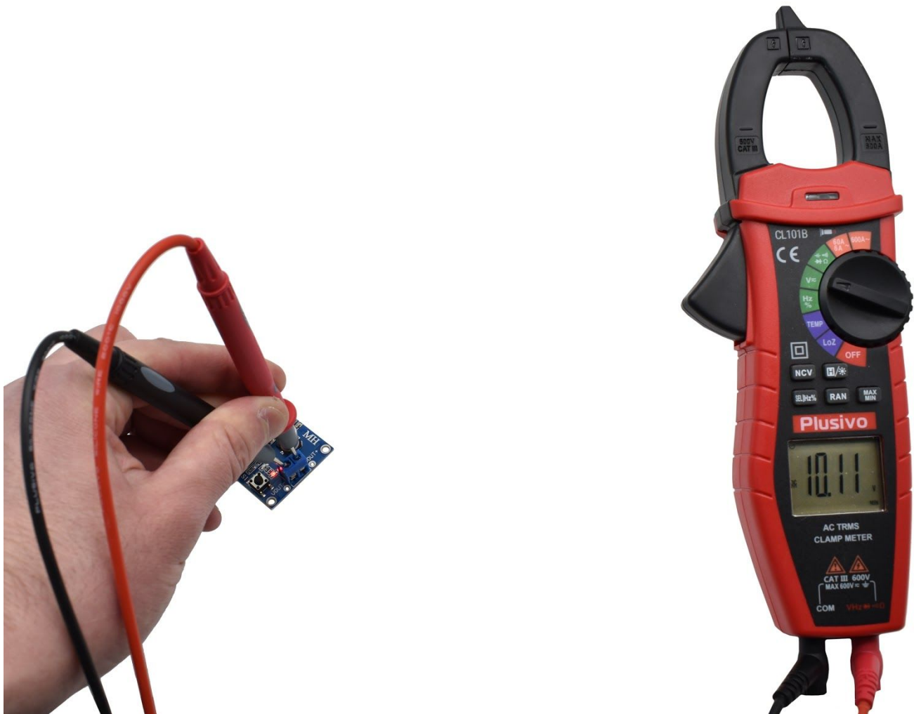
Figure 20. The MIN voltage in this figure is 10.11 V DC.
