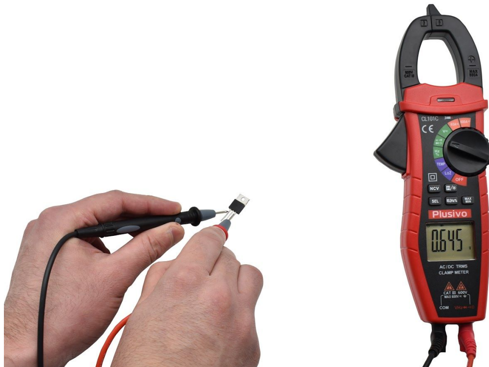
Figure 48. The measured forward voltage in this figure is 0.645 V.
