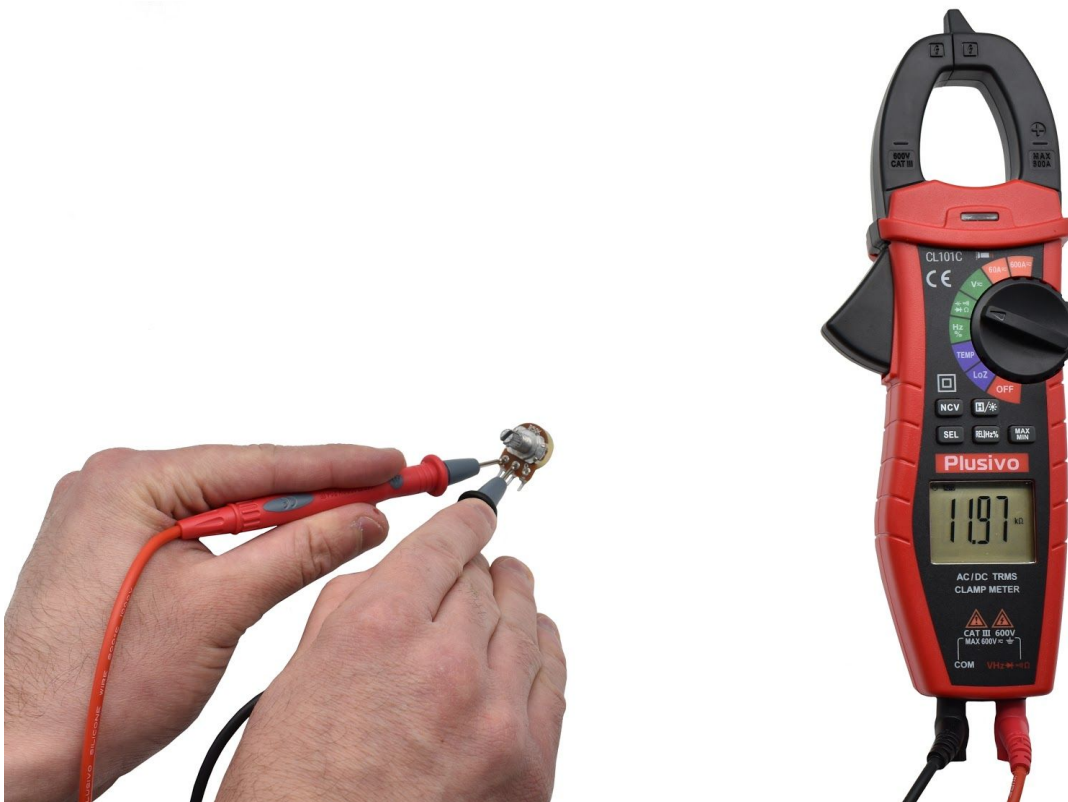
Figure 43. The measured resistance in this figure is 11.97 kΩ.
