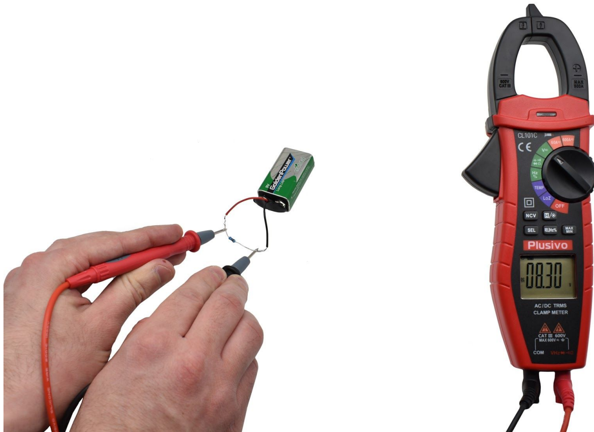
Figure 41. The measured voltage in this figure is 8.30 V DC.
