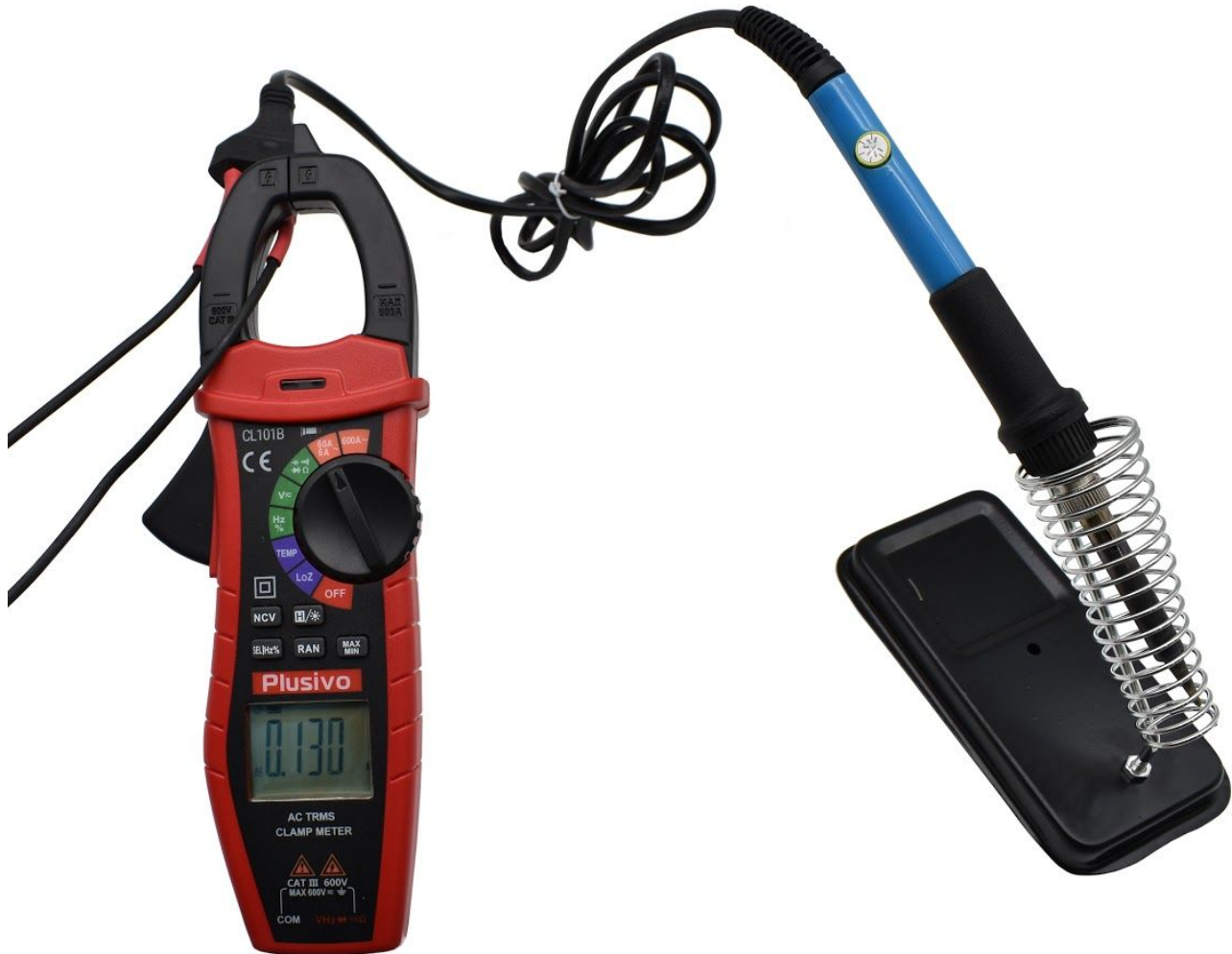
Figure 3. The measured current in this figure is 0.130 A AC.
