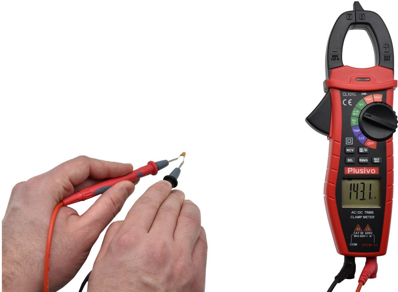
Figure 8. The measured capacitance in this figure is 143.1 nF.
