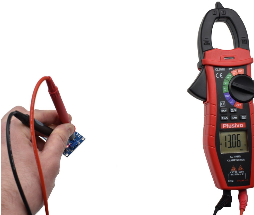
Figure 21. The MAX voltage in this figure is 13.06 V DC.
