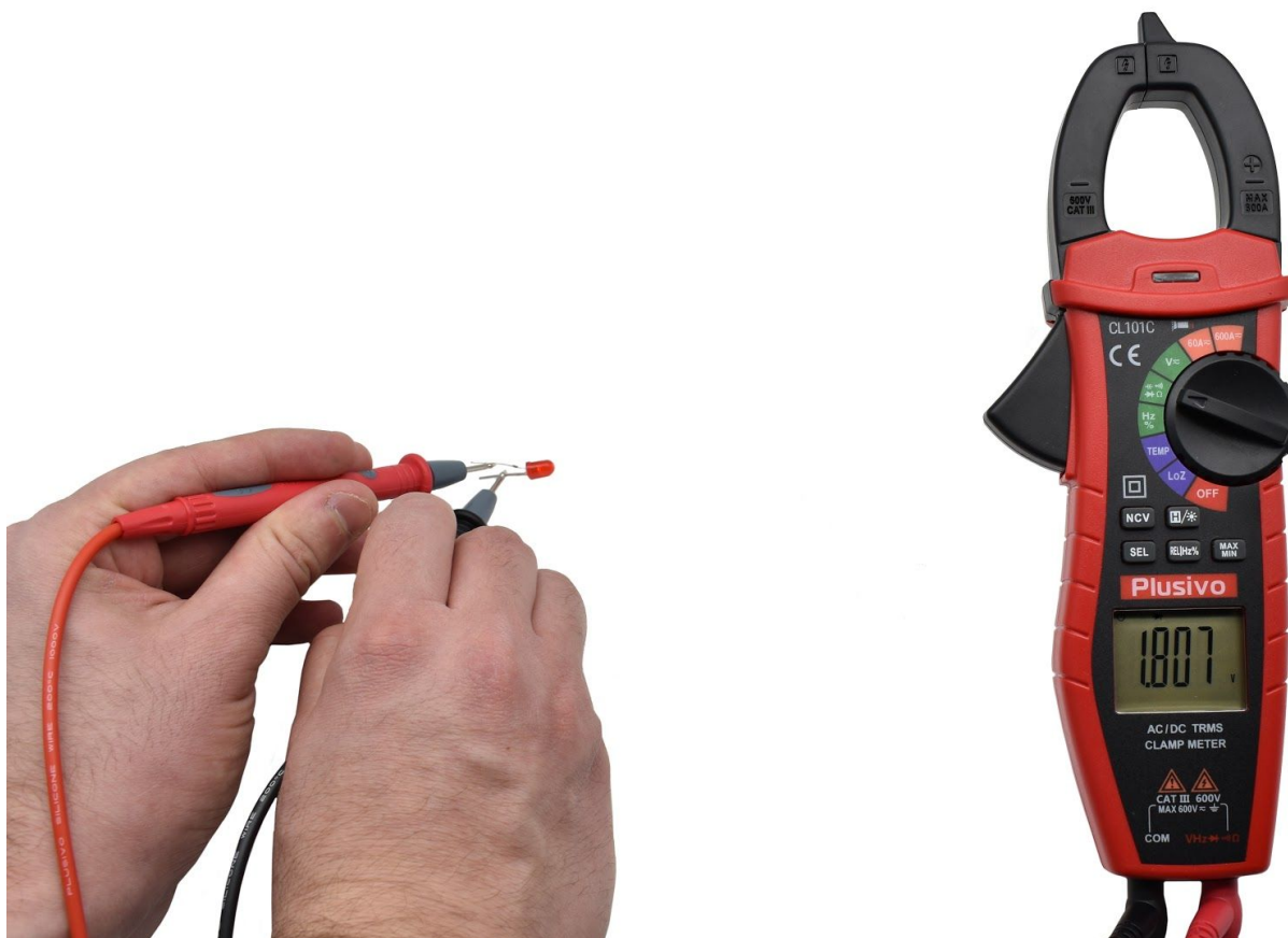
Figure 12. The measured forward voltage in this figure is 1.807 V.
