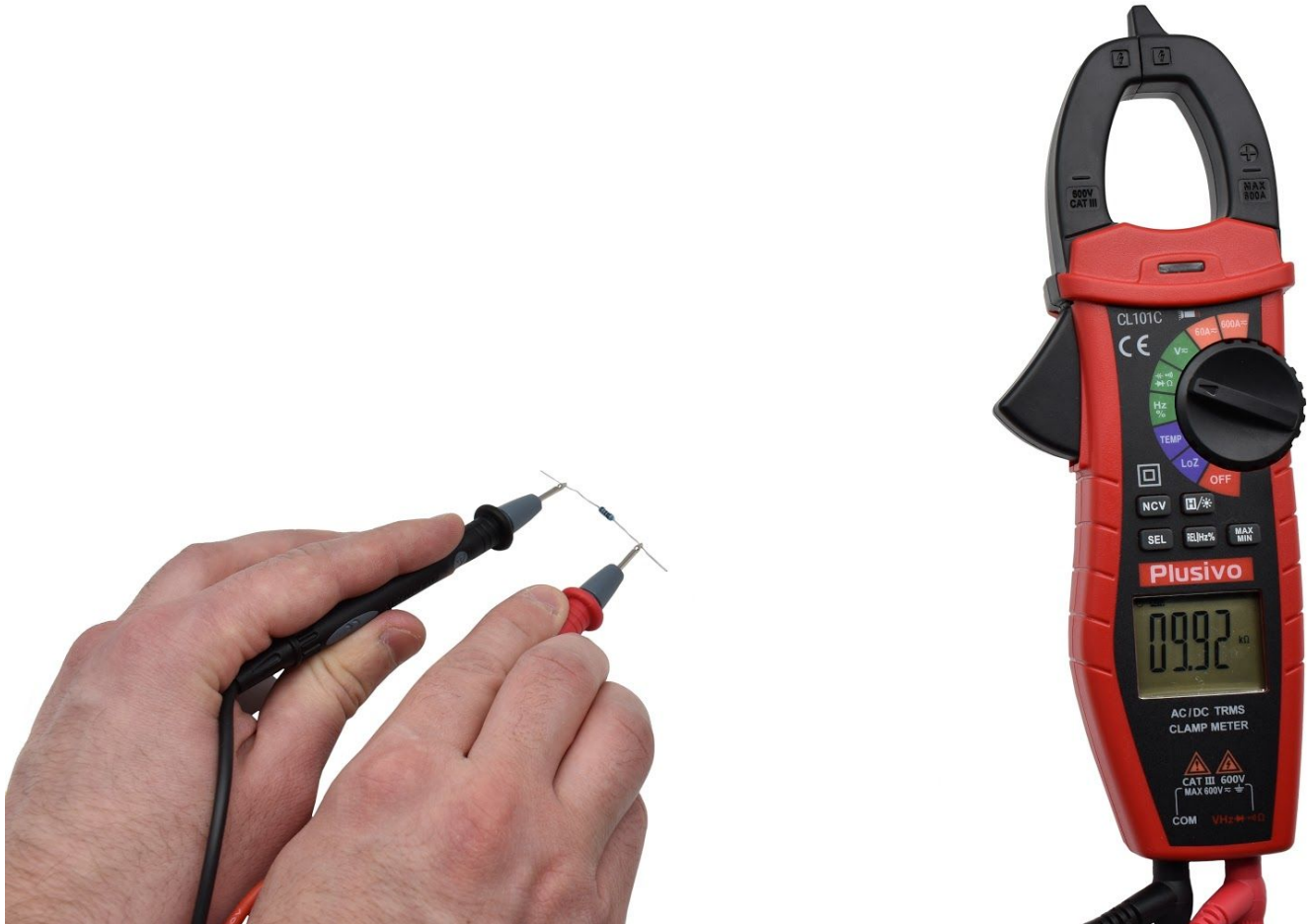
Figure 6. The measured resistance in this figure is 9.92 kΩ.
