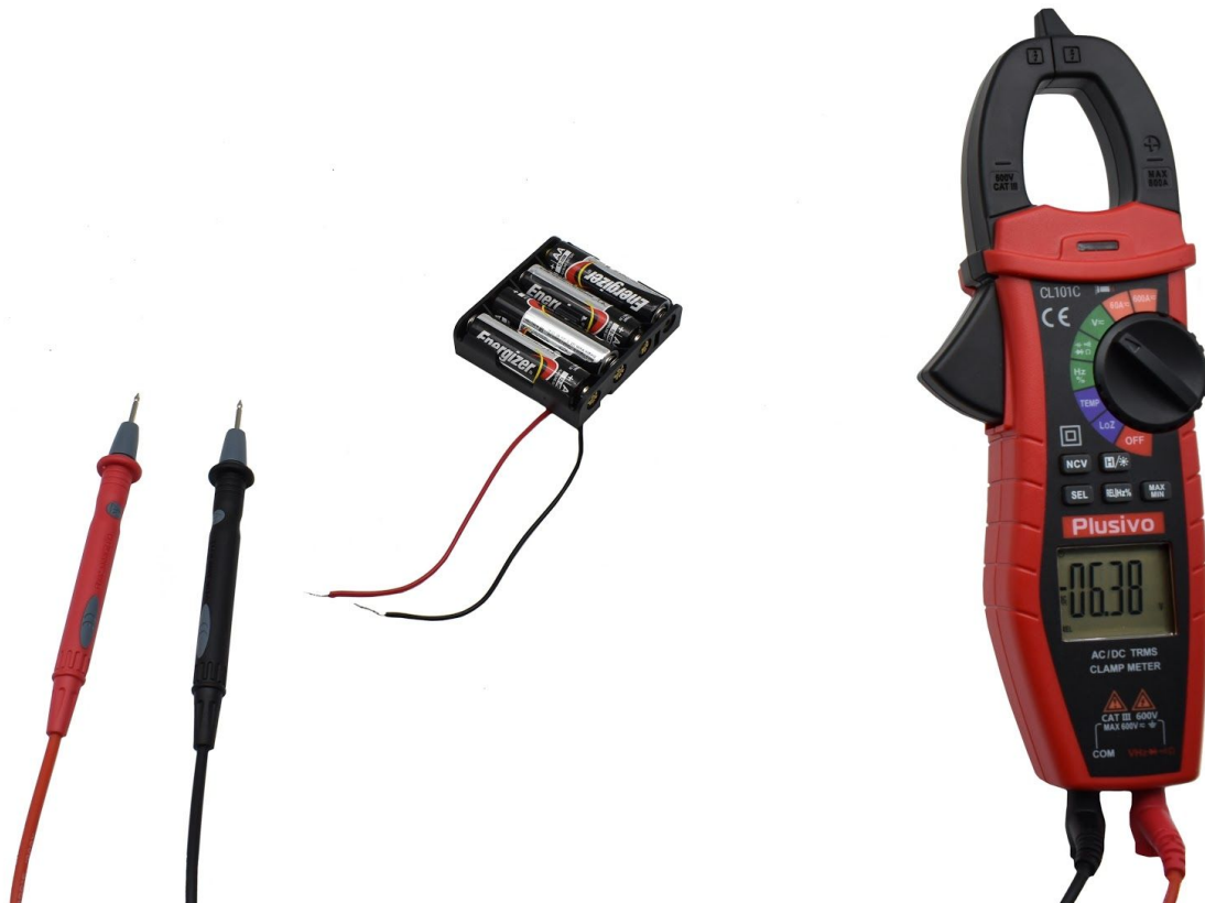
Figure 25. The measured voltage in this figure is -6.38 V DC.
