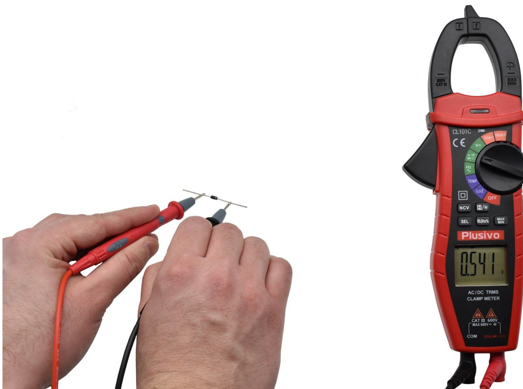
Figure 10. The measured forward voltage in this figure is 0.541 V.
