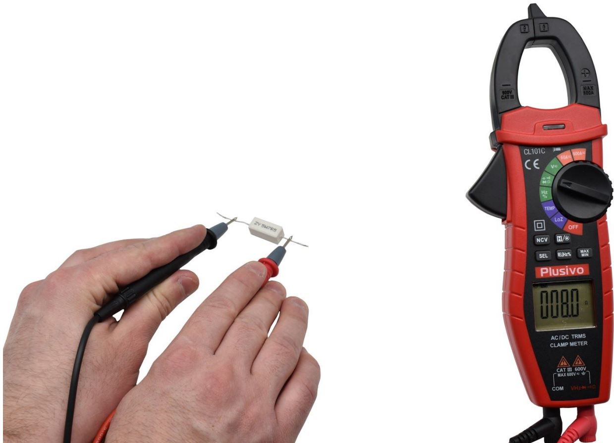
Figure 7. The measured resistance in this figure is 8.0 Ω.
