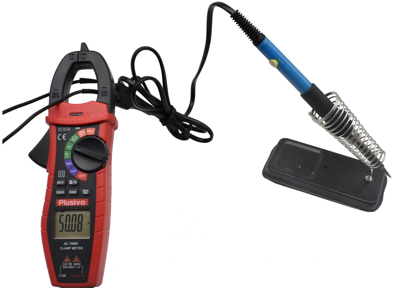
Figure 18. The measured frequency in this figure is 50.08 Hz.
