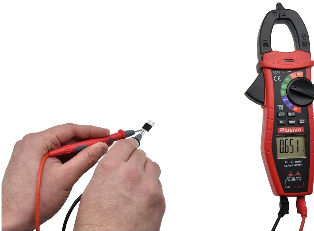
Figure 45. The measured forward voltage in this figure is 0.651 V.
