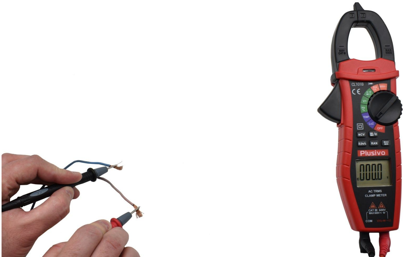
Figure 28. The measured voltage in this figure is 0.0 V AC.
