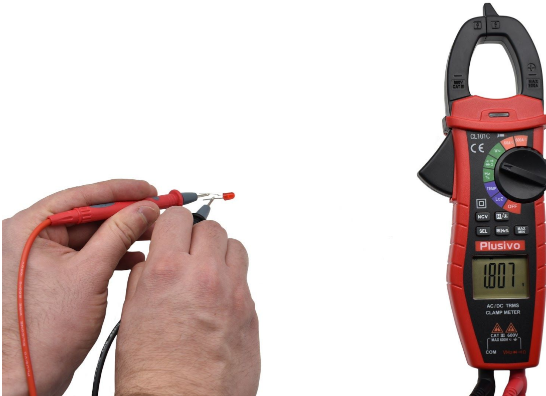
Figure 39. The measured forward voltage in this figure is 1.807 V.
