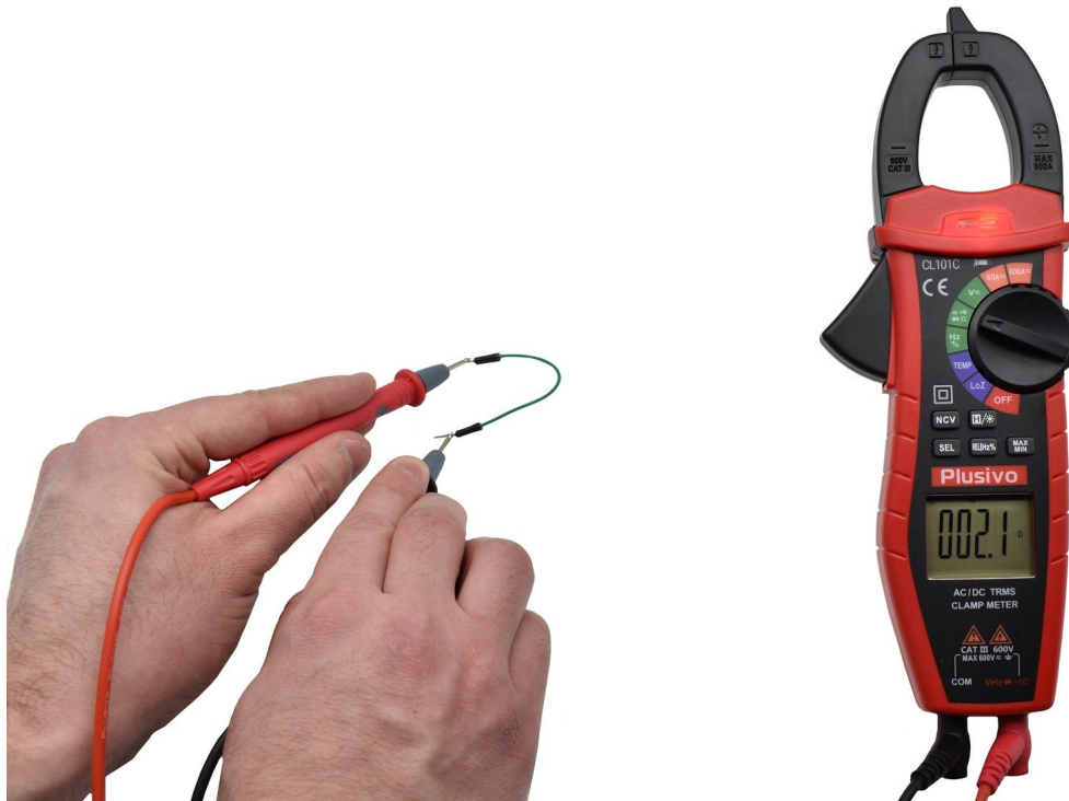
Figure 13. If a conductor path is connected, the clamp meter will beep and the alarm indicator light will light up.
