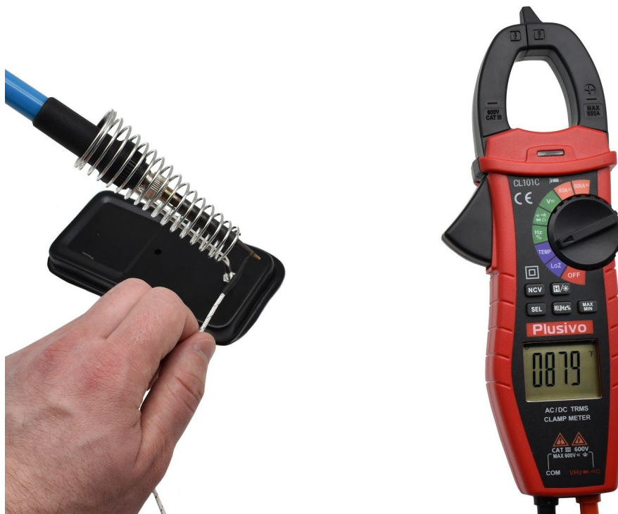
Figure 16. The measured temperature in this figure is 879 °F.
