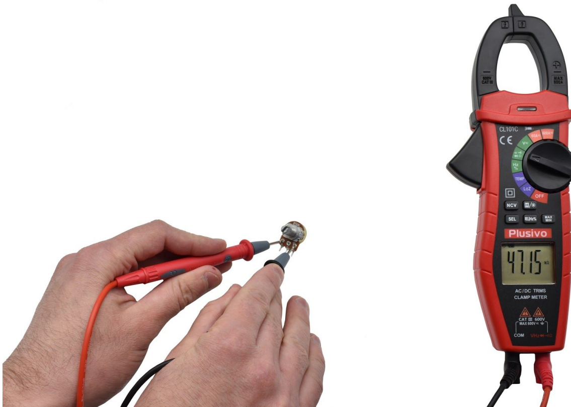
Figure 42. The measured resistance in this figure is 47.15 kΩ.
