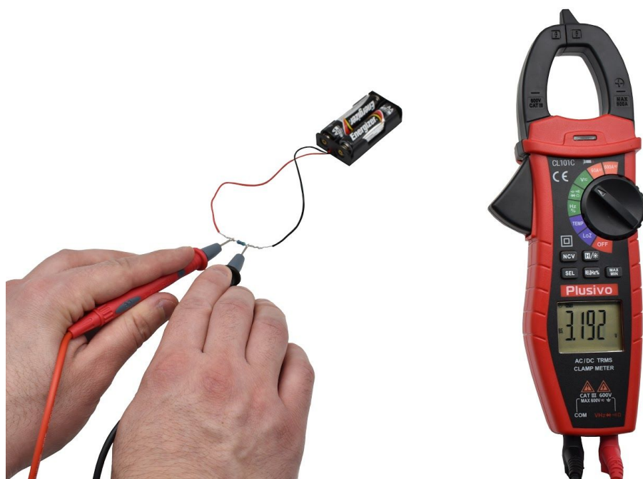
Figure 33. The measured voltage in this figure is 3.192 V DC.
