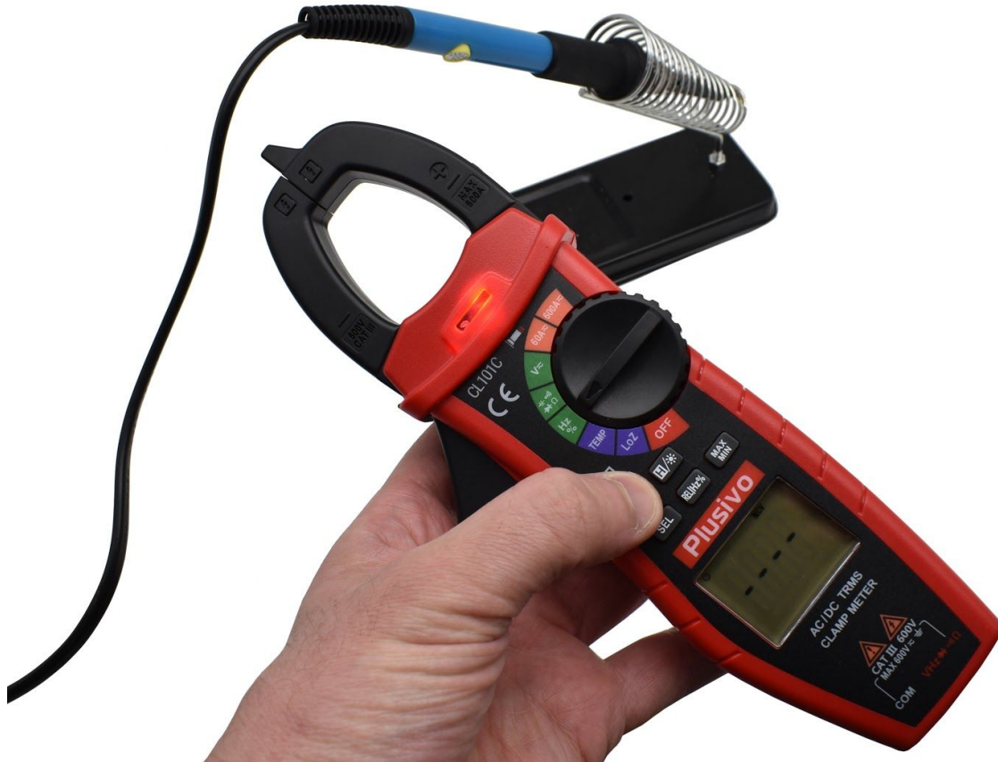
Figure 29. Clamp meter detects AC voltage.
