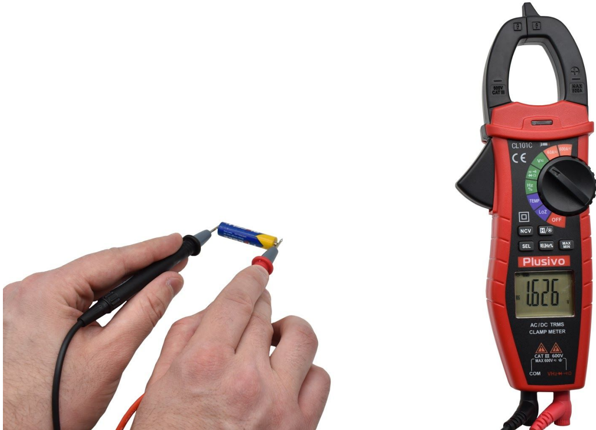
Figure 1. The measured voltage in this figure is 1.626 V DC.
