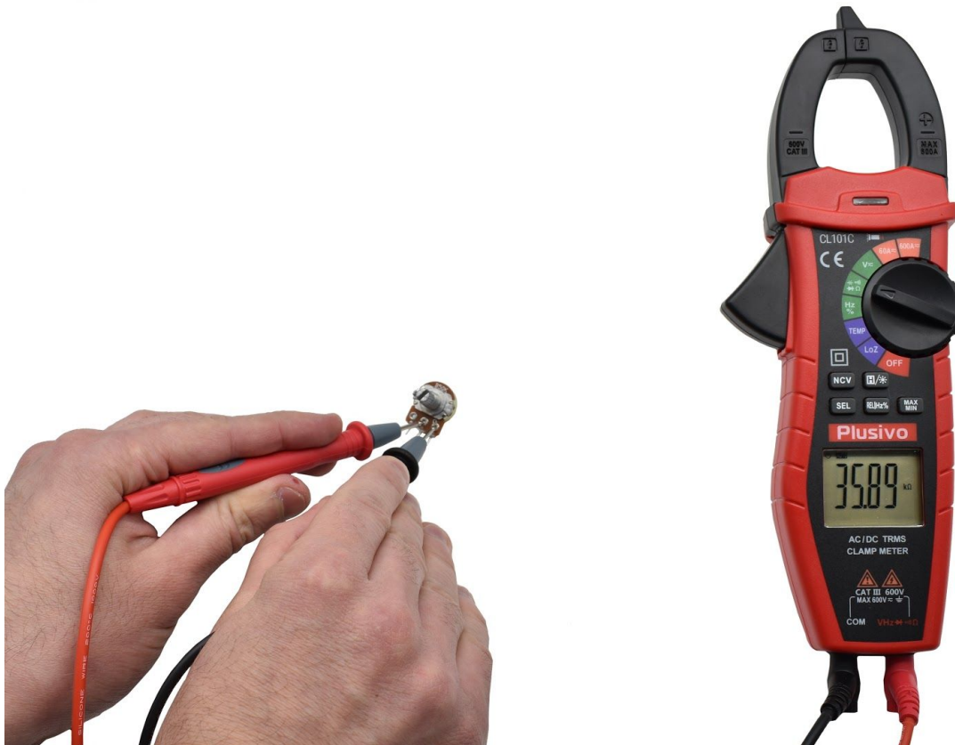
Figure 44. The measured resistance in this figure is 35.89 kΩ.
