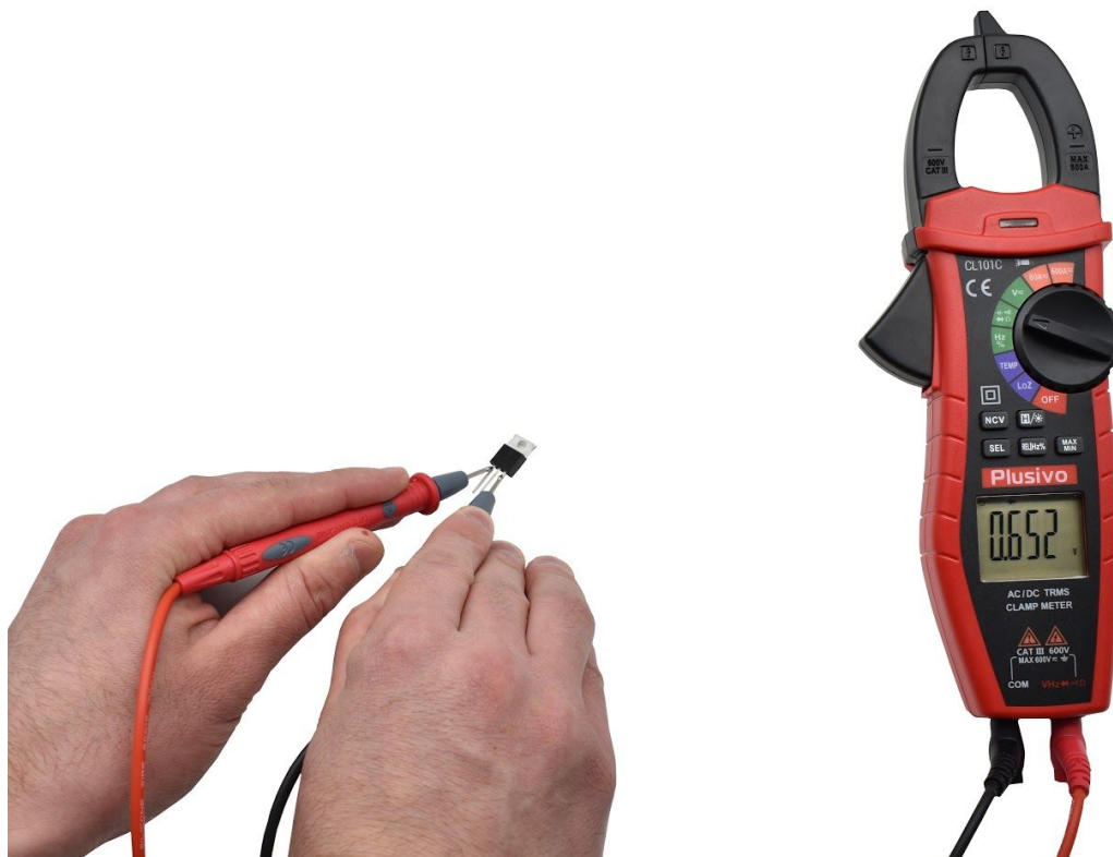
Figure 46. The measured forward voltage in this figure is 0.652 V.
