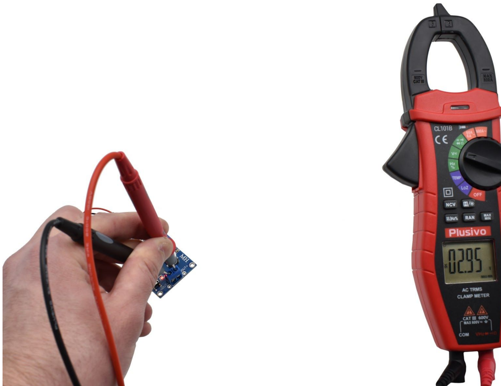
Figure 22. The MAX-MIN voltage in this figure is 2.95 V DC.
