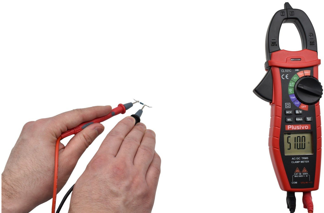
Figure 30. The measured resistance in this figure is 510 Ω.
