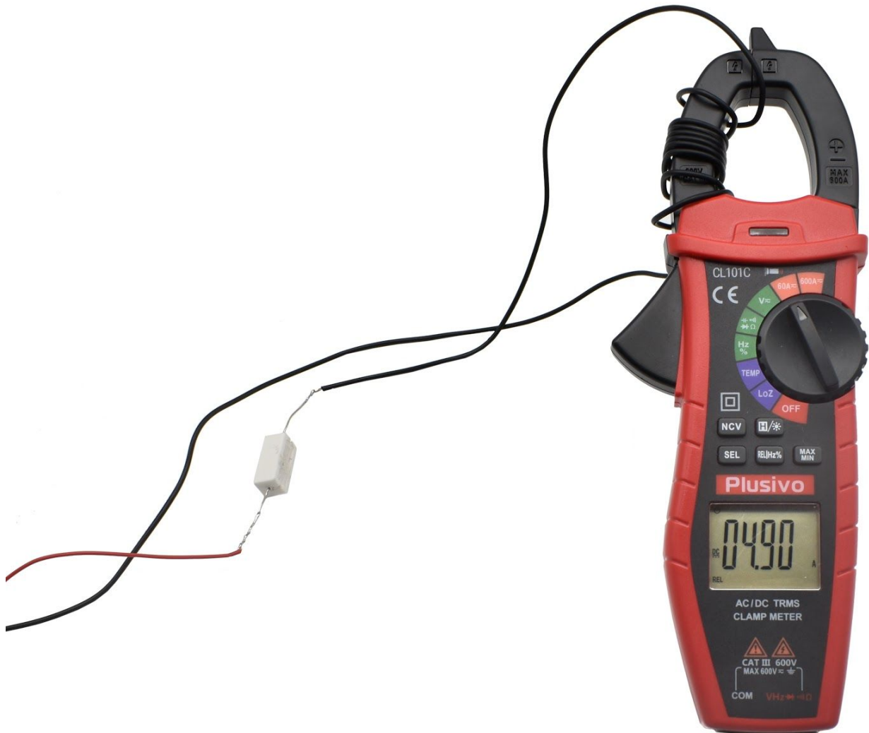
Figure 5. The measured current in this figure is 4.90 A DC.
