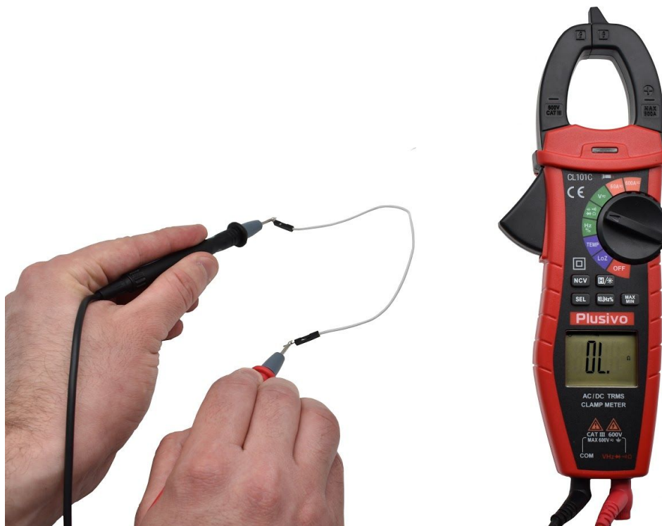
Figure 14. If a conductor path is broken the clamp meter will not beep.
