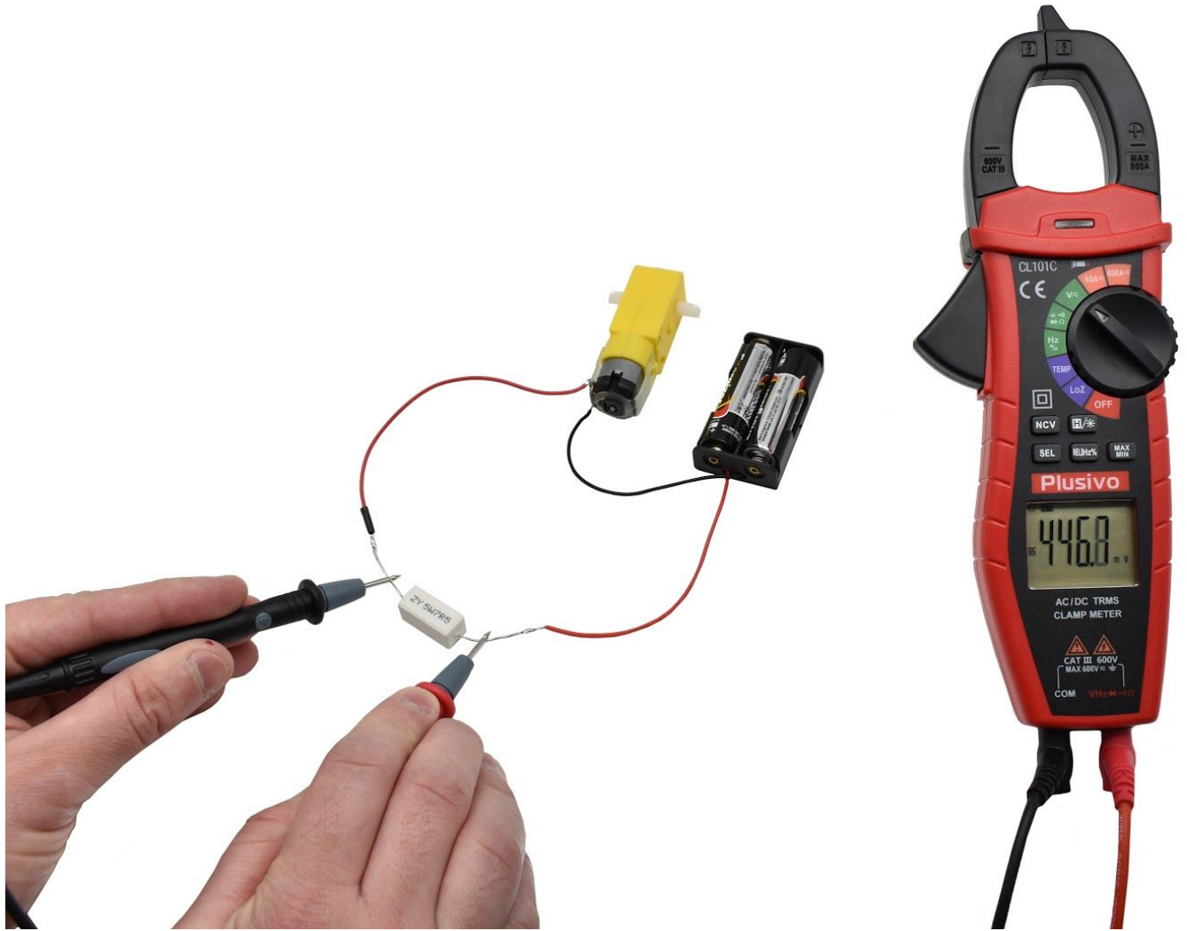
Figure 38. The measured voltage in this figure is 446.7 mV DC.
