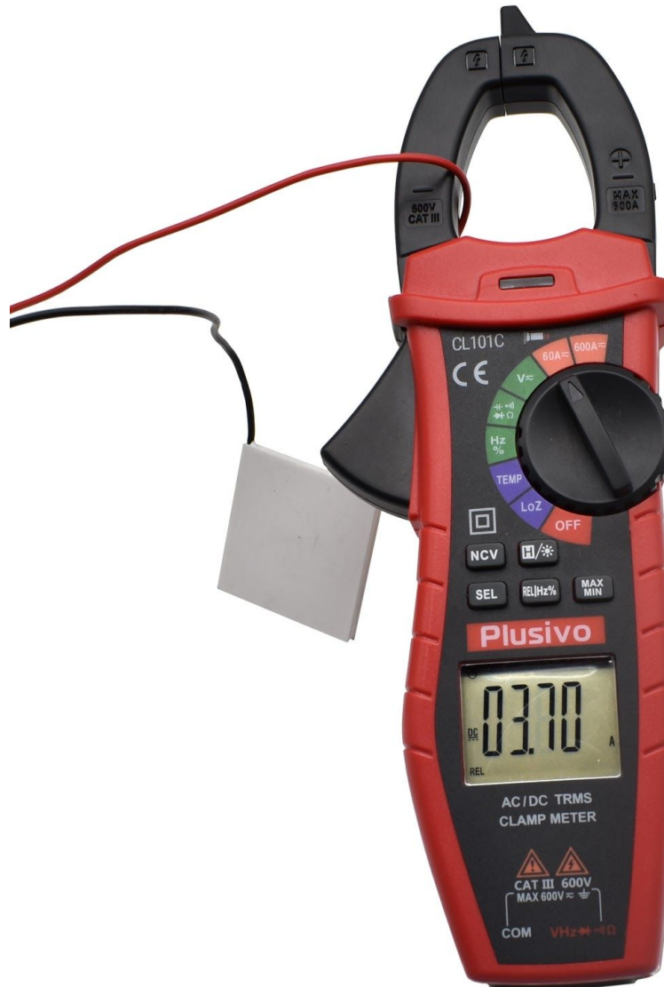
Figure 4. The measured current in this figure is 3.70 A DC.
