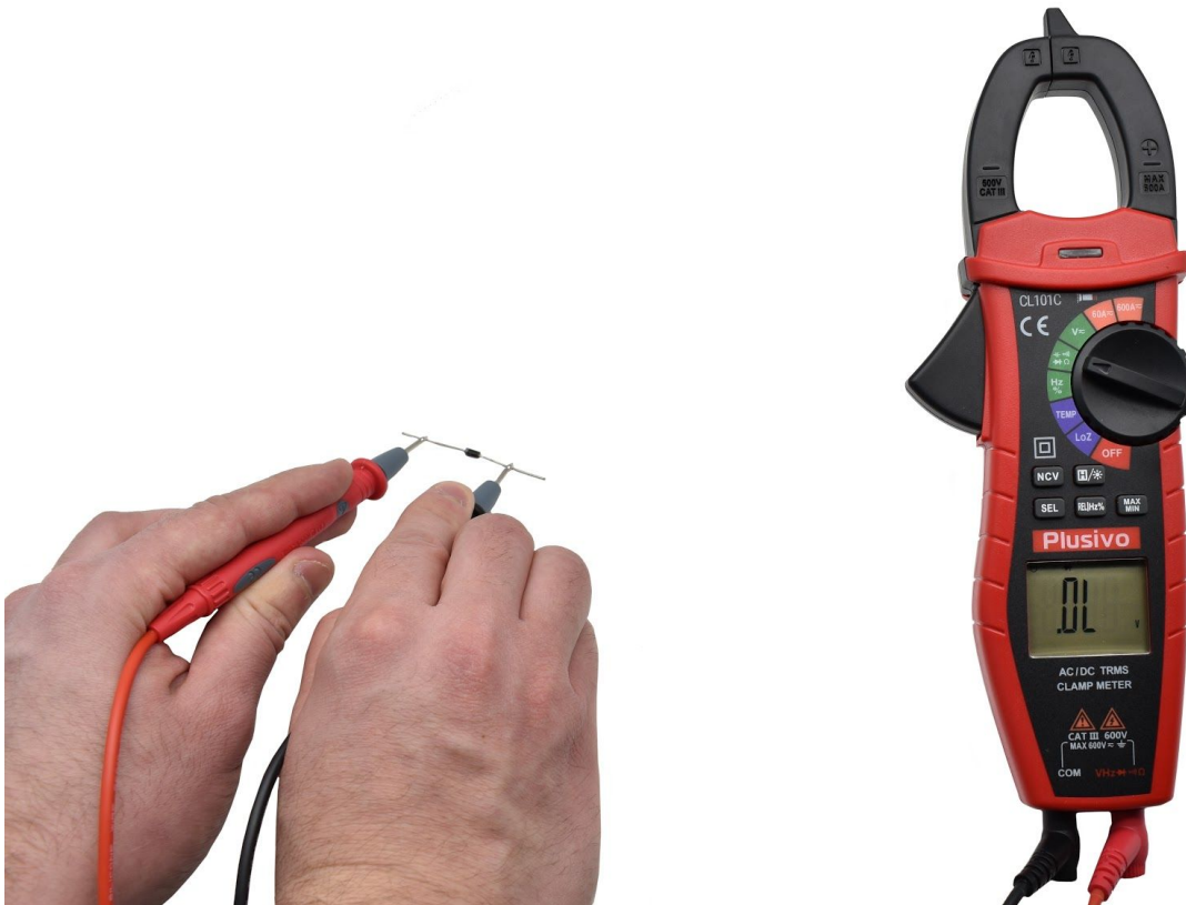
Figure 11. If you connect the probes incorrectly, the display will show "OL".
