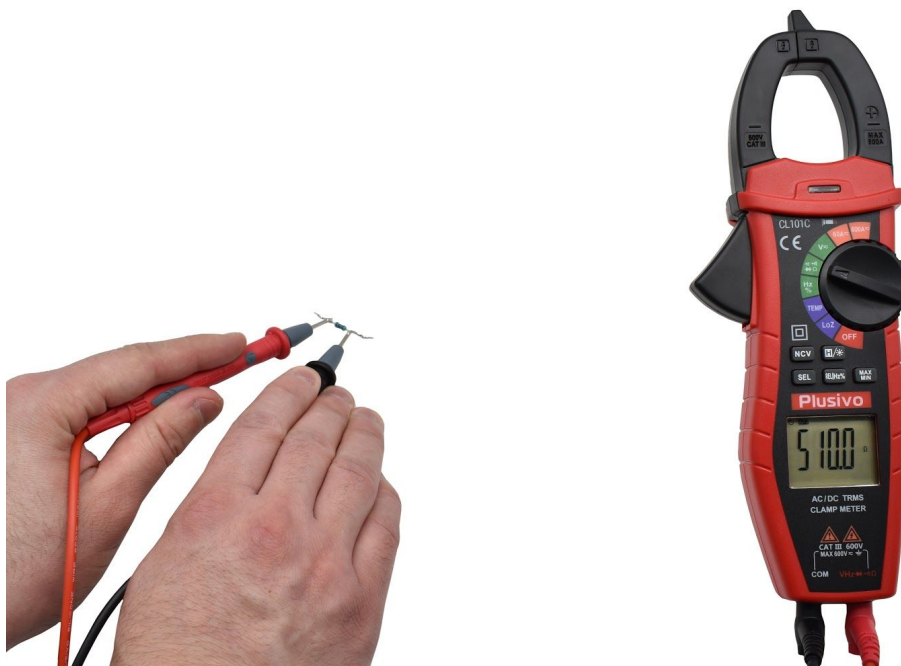
Figure 32. The measured resistance in this figure is 510 Ω.
