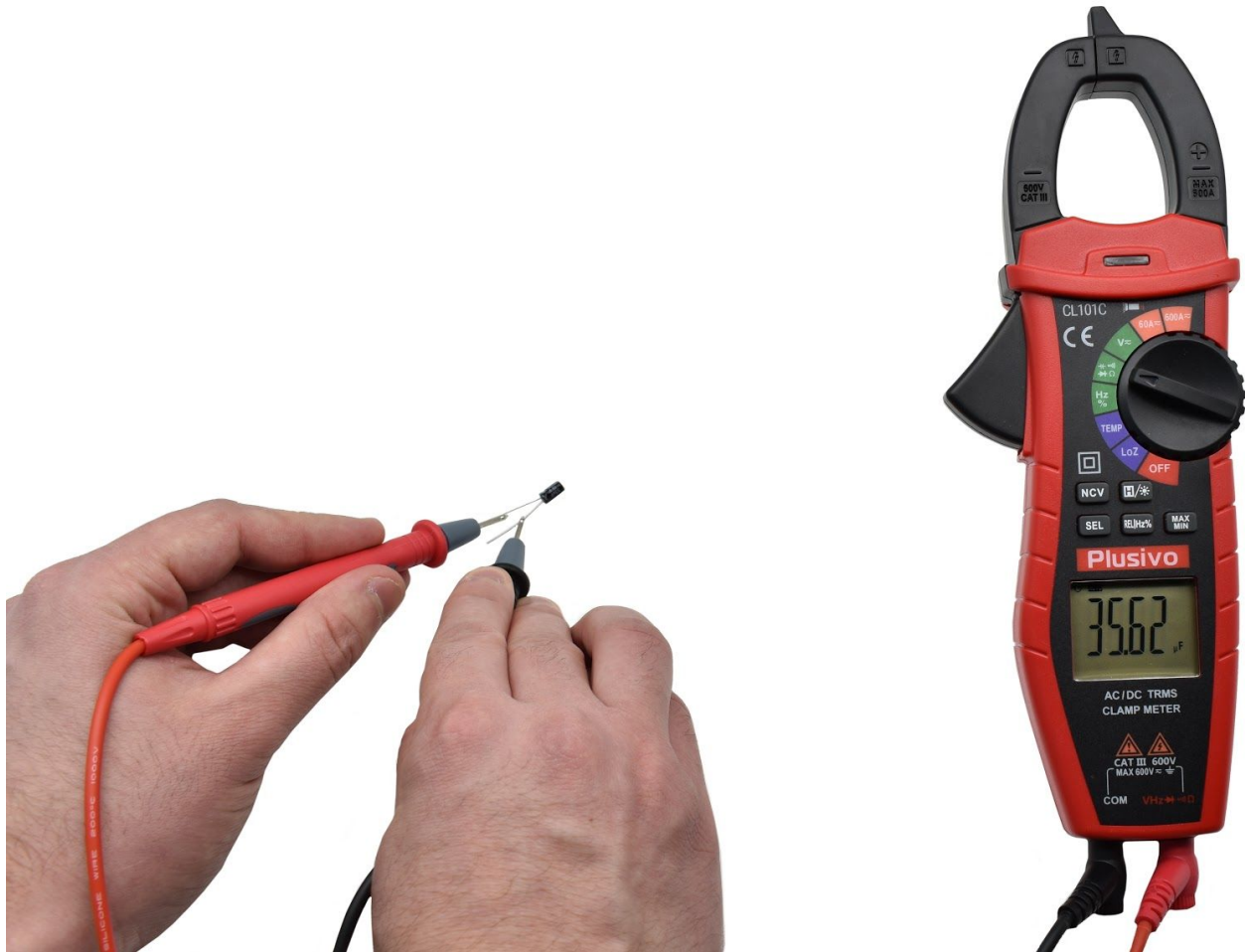
Figure 9. The measured capacitance in this figure is 35.62 \mu\text{F} .
