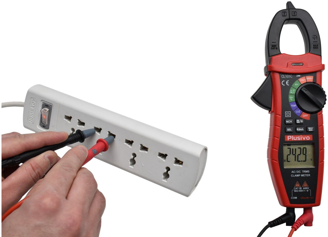
Figure 2. The measured voltage in this figure is 242.9 V AC.
