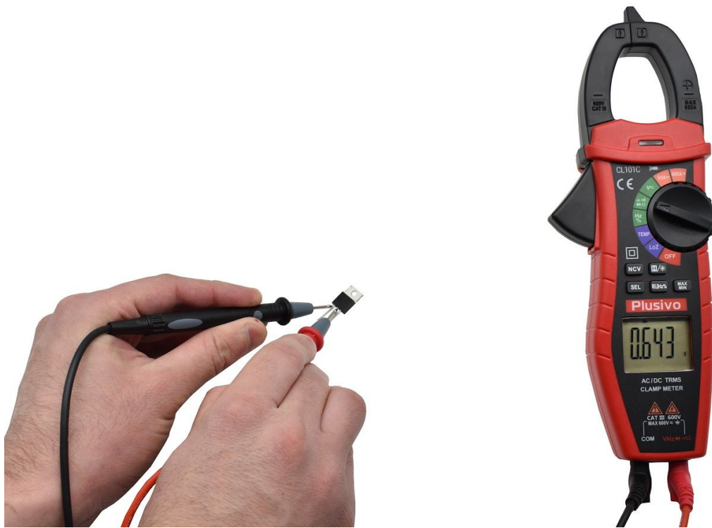
Figure 47. The measured forward voltage in this figure is 0.643 V.
