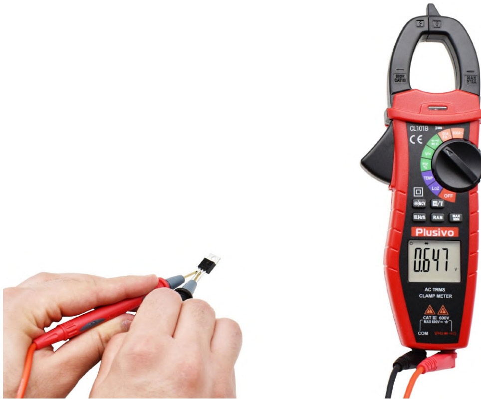
Figure 45. The measured forward voltage in this figure is 0.647 V
