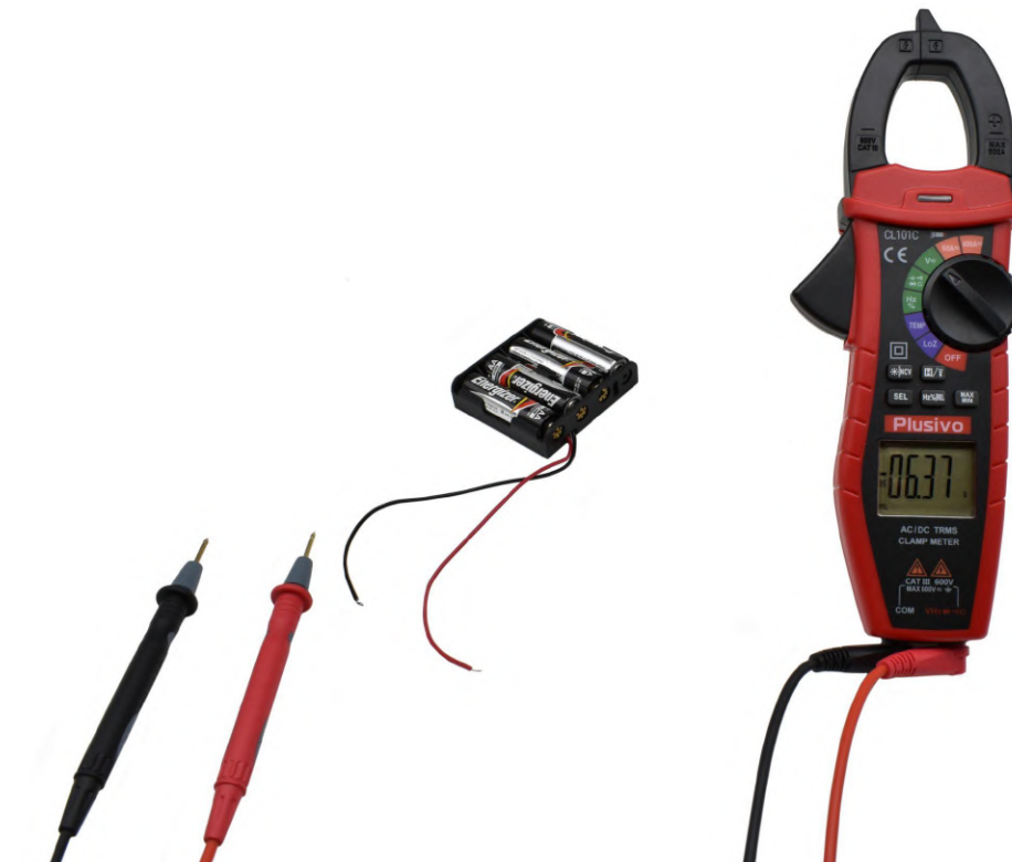
Figure 25. The measured voltage in this figure is -6.37 V DC
