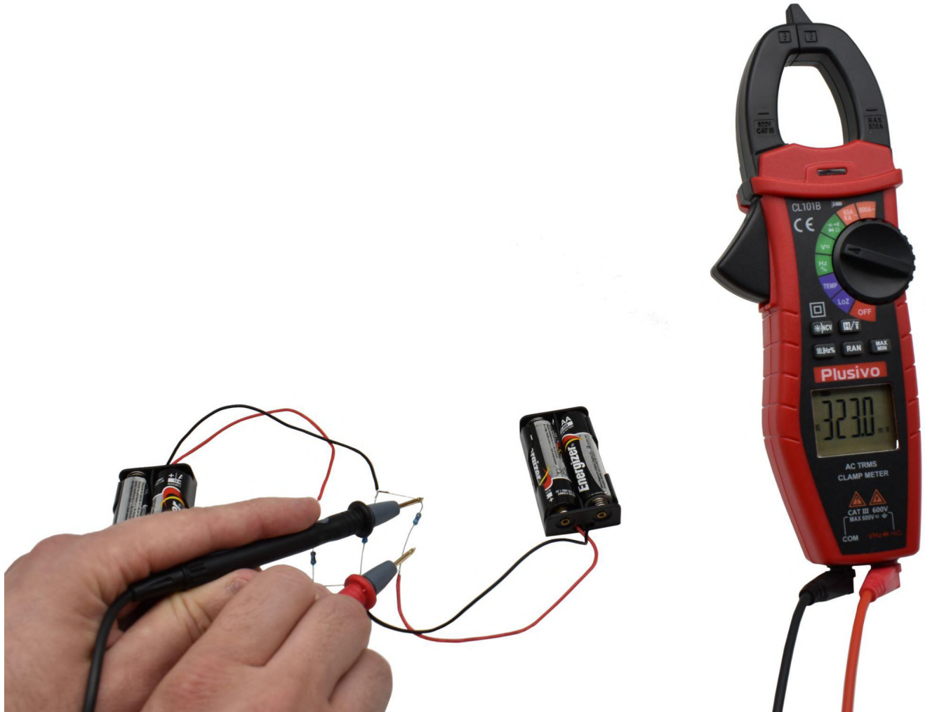
Figure 36. The measured voltage in this figure is 323.0 mV DC
