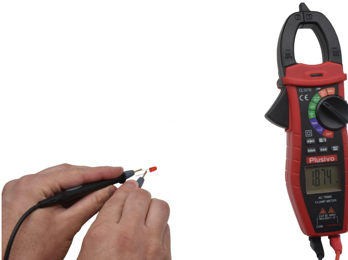
Figure 12. The measured forward voltage in this figure is 1.874 V
