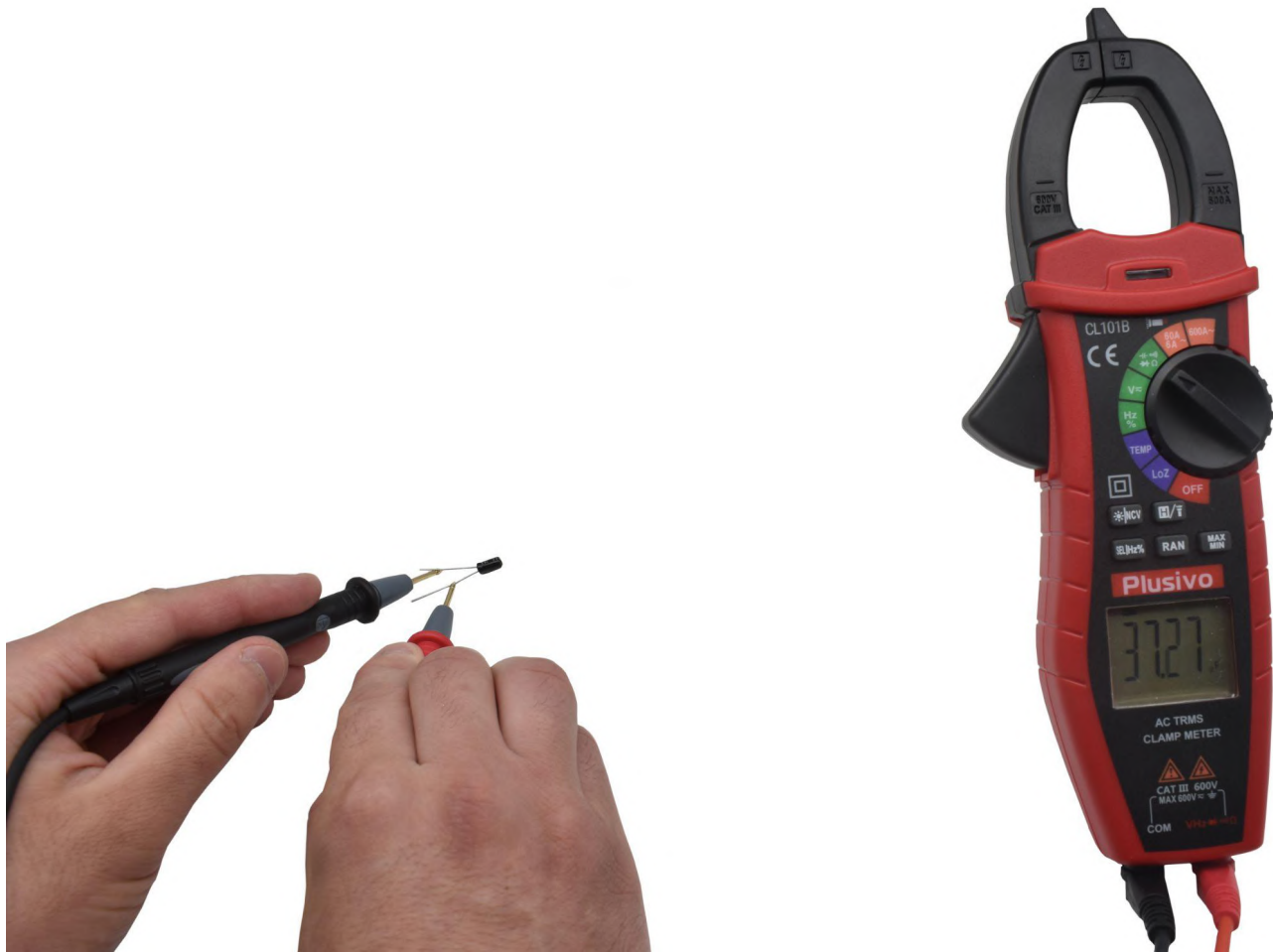
Figure 9. The measured capacitance in this figure is 37.27 \mu F
