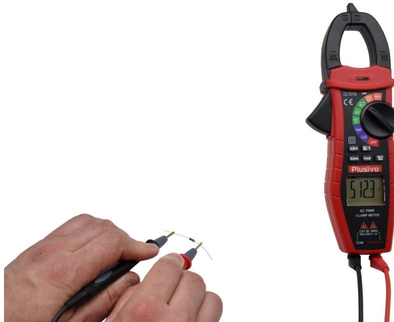
Figure 32. The measured resistance in this figure is 512.3 \Omega
