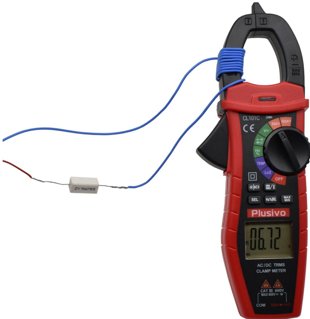
Figure 5. The measured current in this figure is 6.72 A DC
