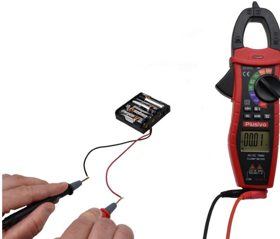
Figure 24. The measured voltage in this figure is 0.01 V DC
