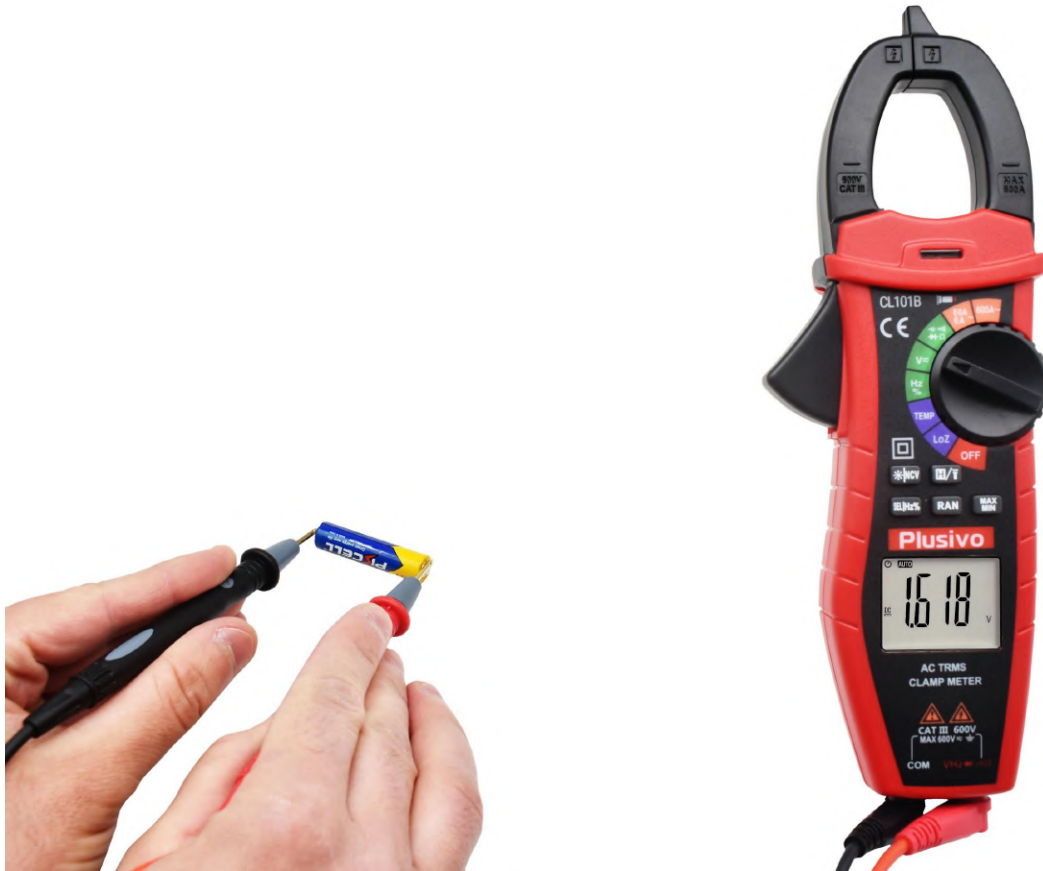
Figure 1. The measured voltage in this figure is 1.618 V DC
