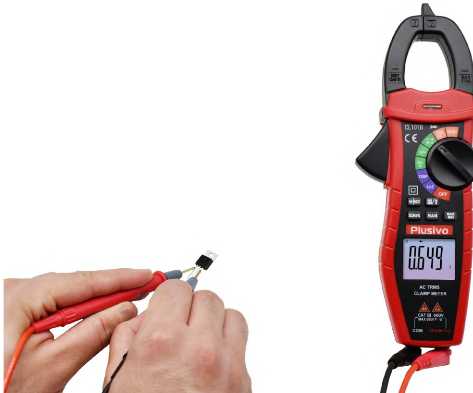
Figure 46. The measured forward voltage in this figure is 0.649 V
