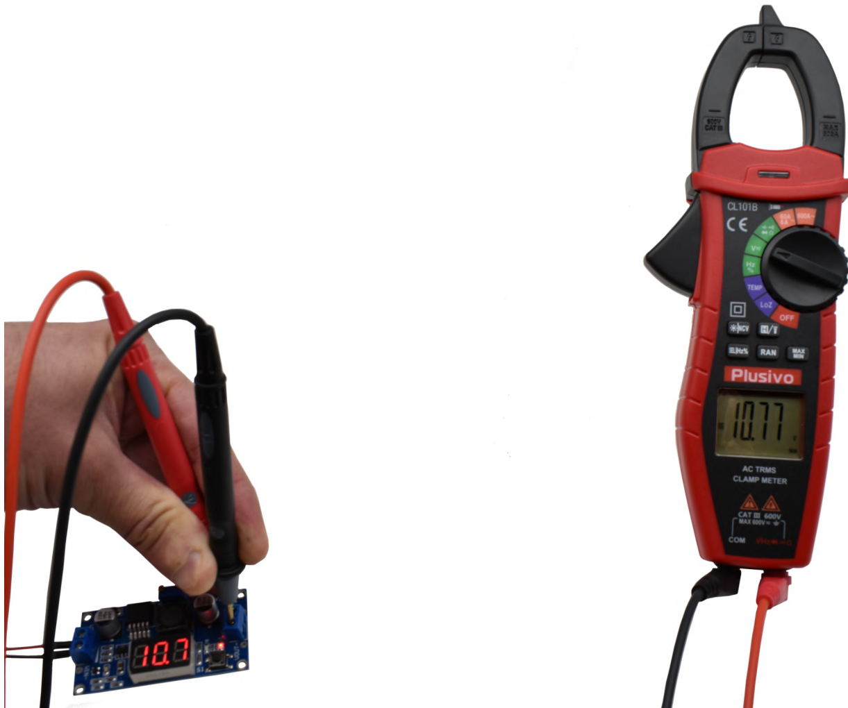
Figure 20. The MIN voltage in this figure is 10.77 V DC
