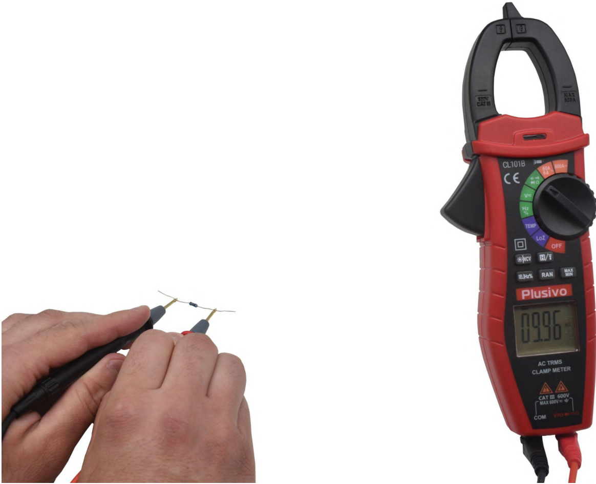
Figure 6. The measured resistance in this figure is 9.96 k \Omega
