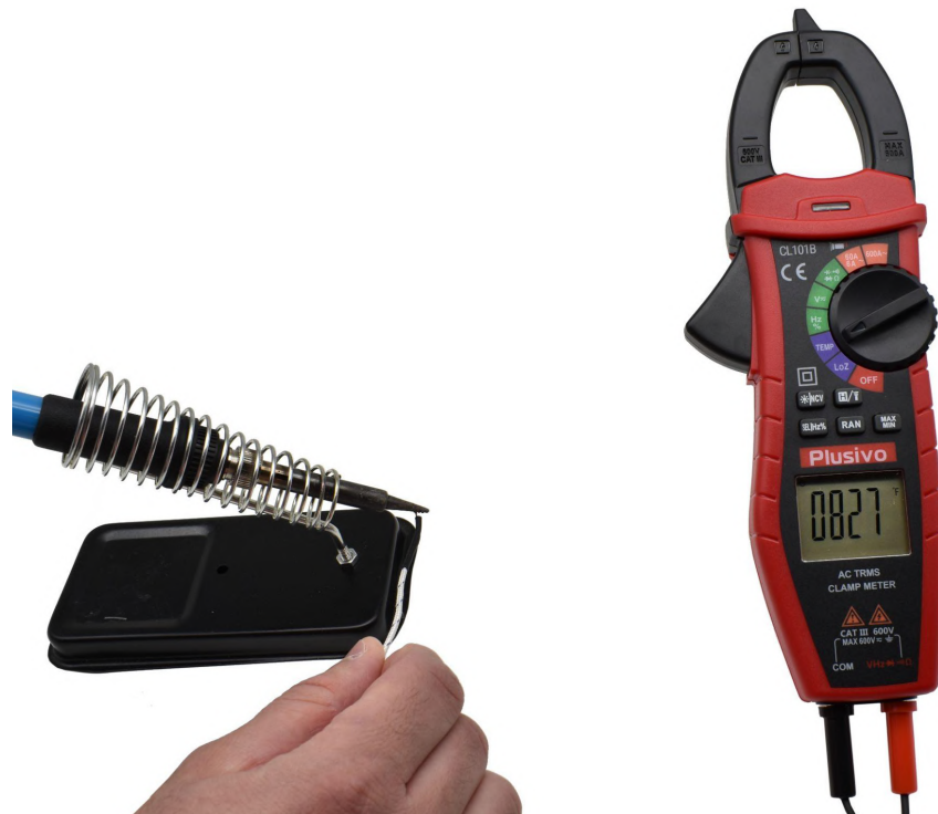
Figure 16. The measured temperature in this figure is 827 °F
