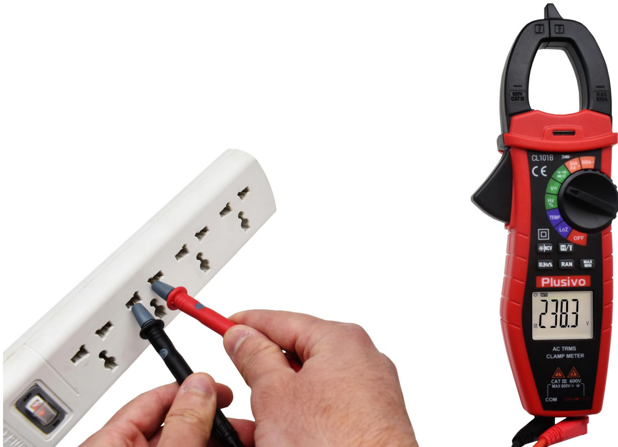
Figure 2. The measured voltage in this figure is 238.3 V AC
