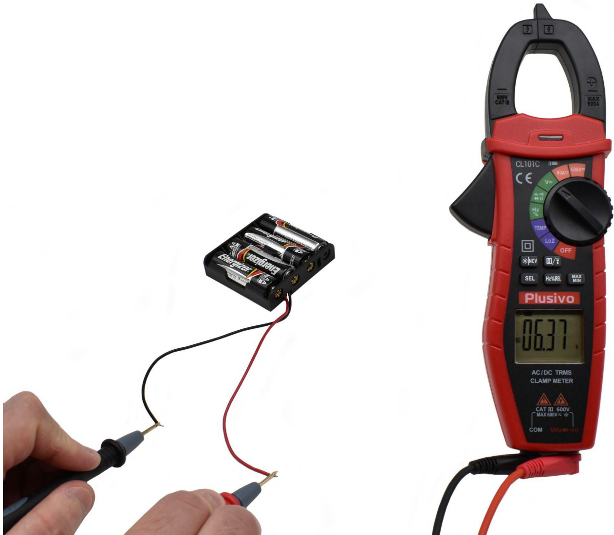
Figure 23. The measured voltage in this figure is 6.37 V DC
