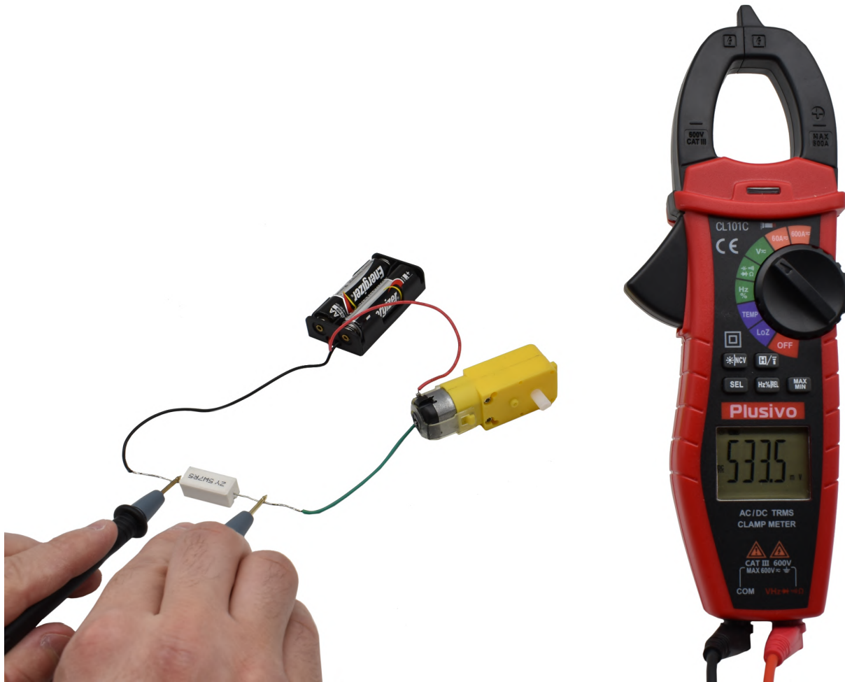
Figure 38. The measured voltage in this figure is 533.5 mV DC
