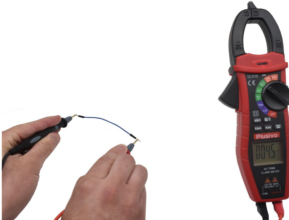
Figure 13. If a conductor path is connected, the clamp meter will beep and the alarm indicator light will light up
