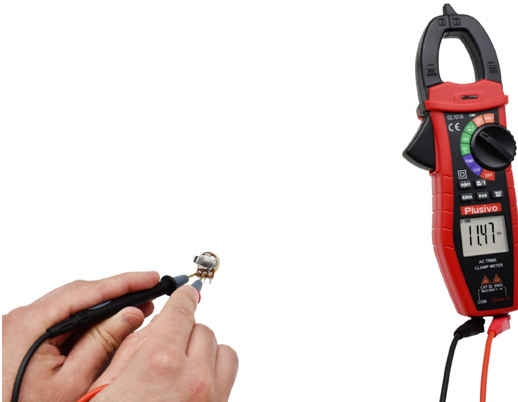
Figure 43. The measured resistance in this figure is 11.47 kΩ
