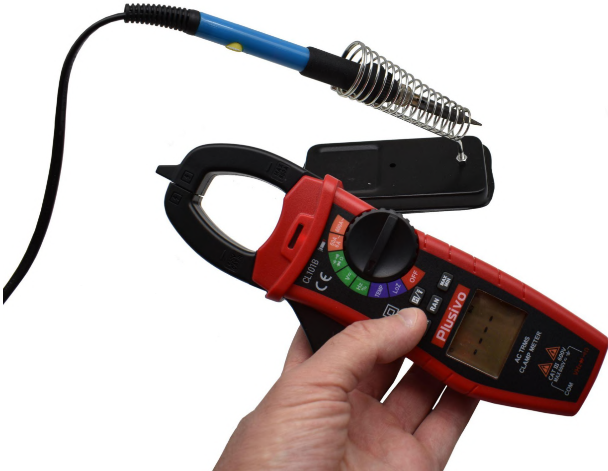
Figure 29. Clamp meter detects AC voltage.
