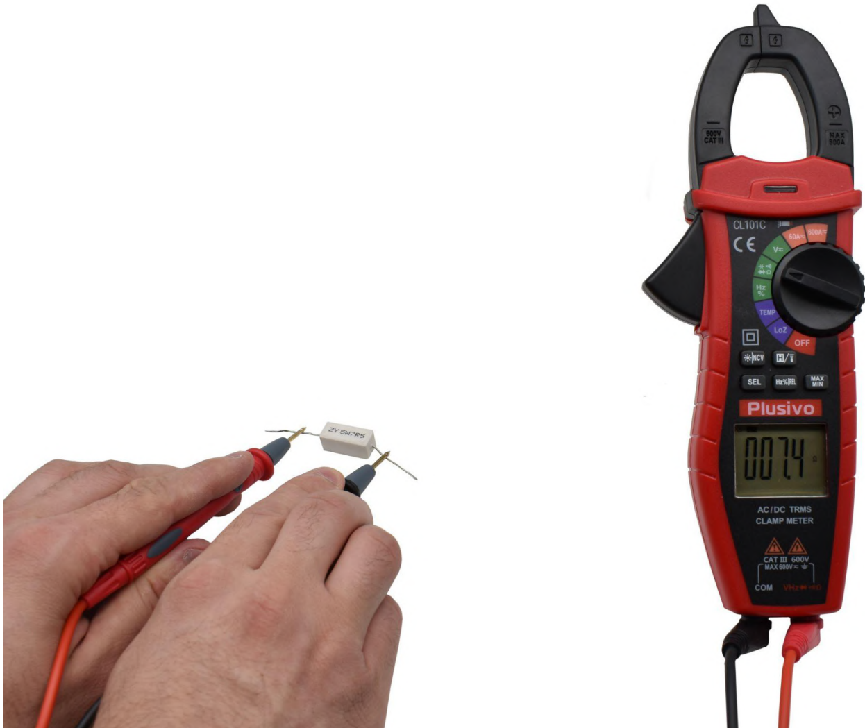
Figure 37. The measured resistance in this figure is 7.4\ \Omega
