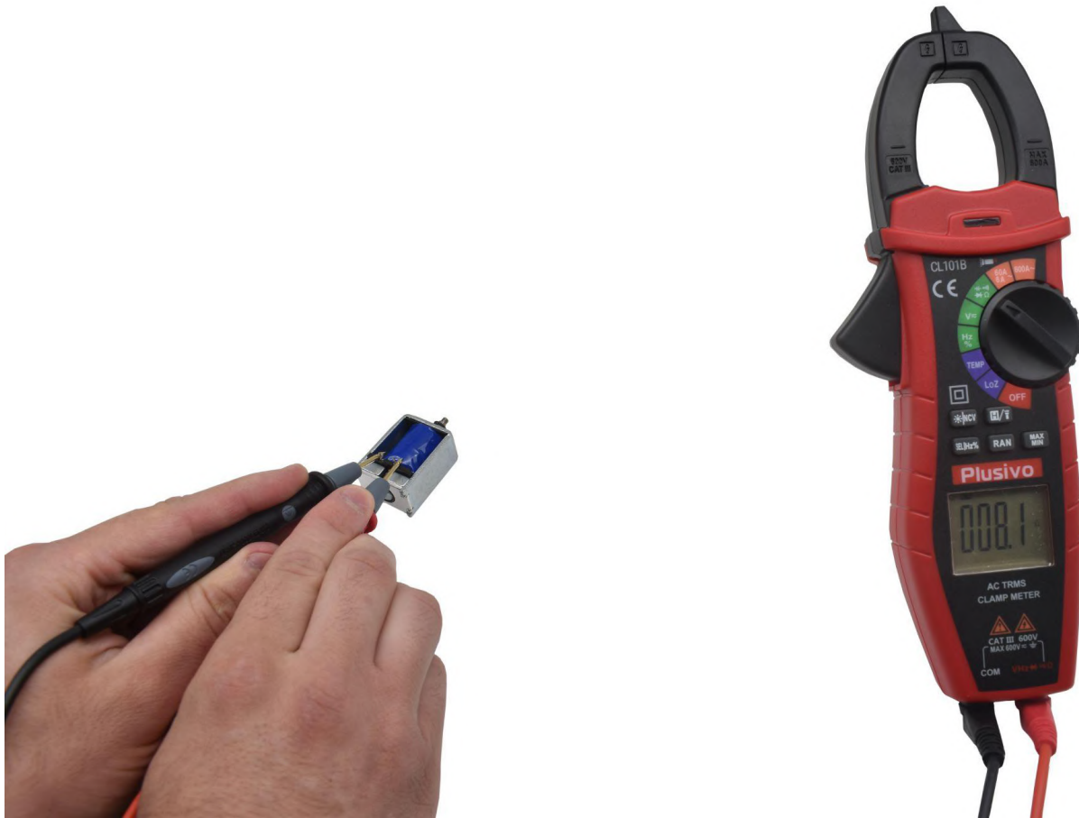
Figure 7. The measured resistance in this figure is 8.1 \Omega
