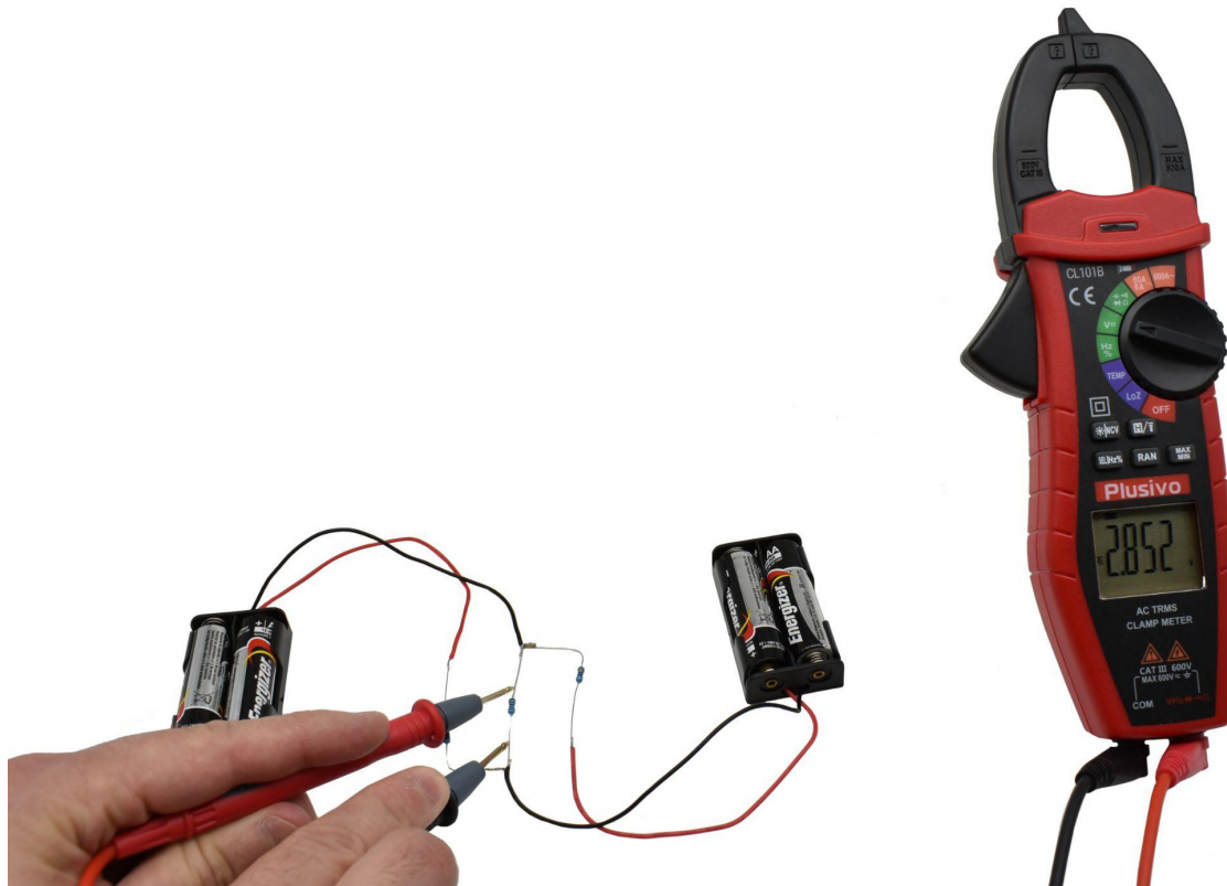
Figure 35. The measured voltage in this figure is 2.852 V DC
