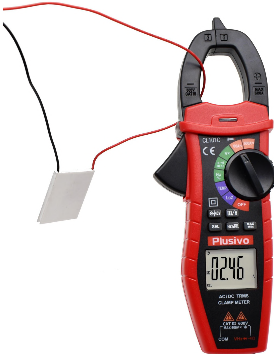
Figure 4. The measured current in this figure is 2.46 A DC
