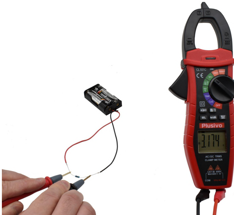
Figure 33. The measured voltage in this figure is 3.174 V DC
