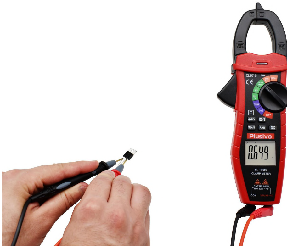
Figure 48. The measured forward voltage in this figure is 0.649 V
