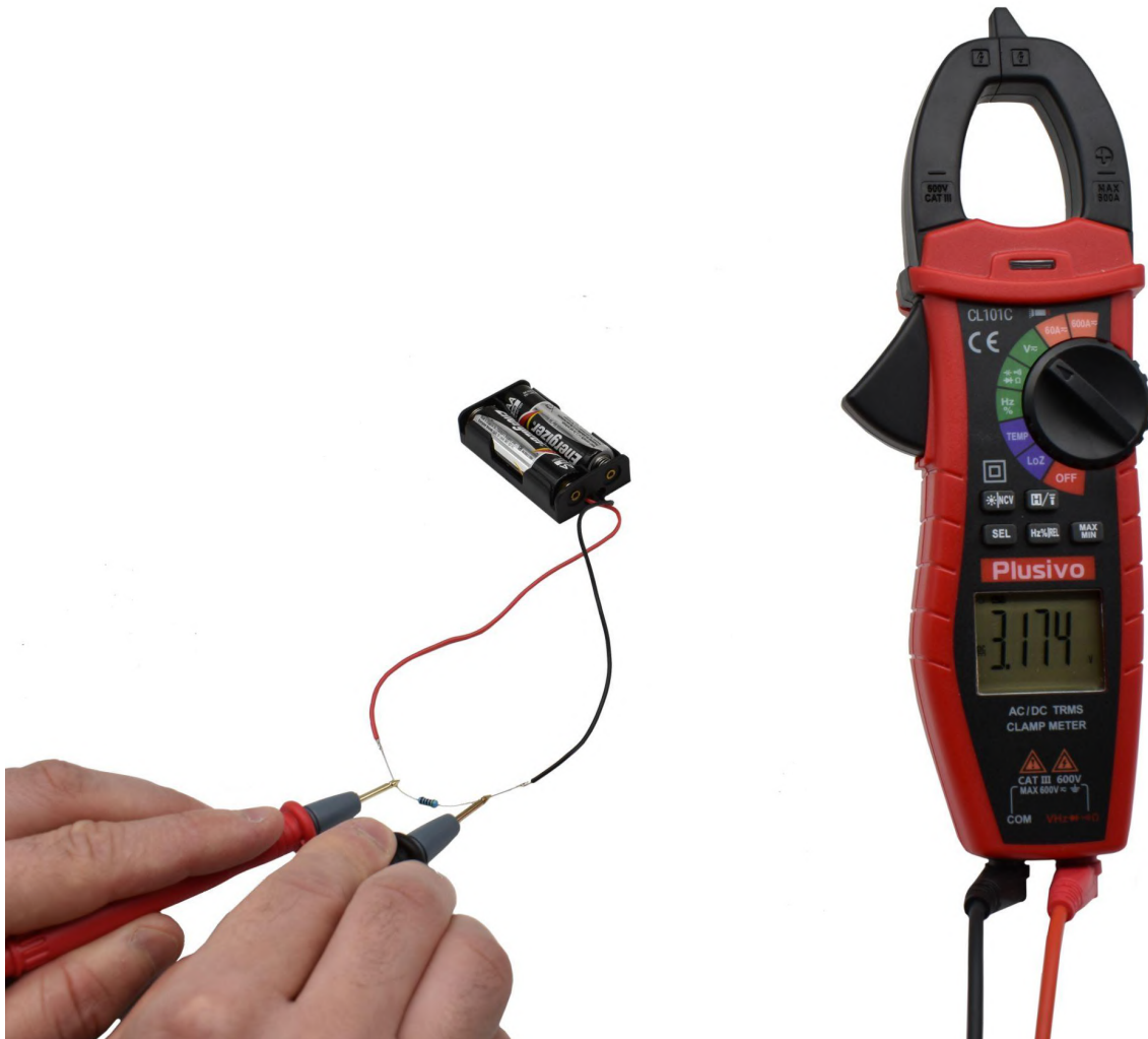
Figure 31. The measured voltage in this figure is 3.174 V DC
