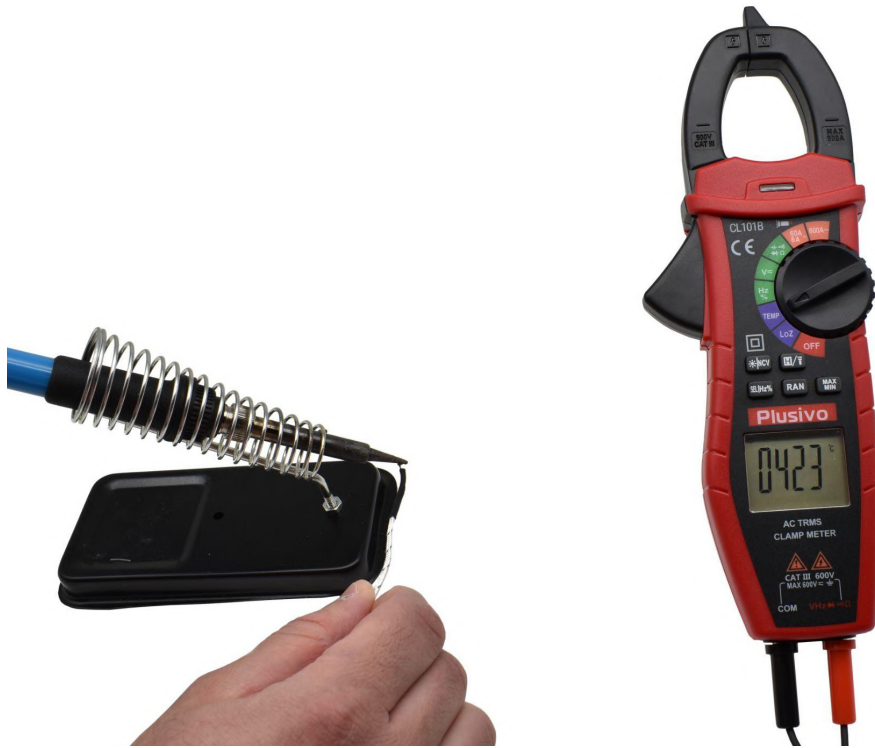
Figure 15. The measured temperature in this figure is 423 °C
