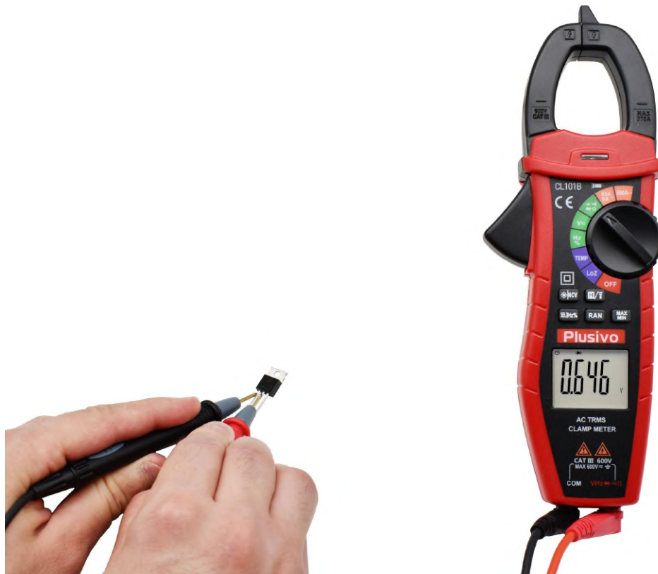
Figure 47. The measured forward voltage in this figure is 0.646 V
