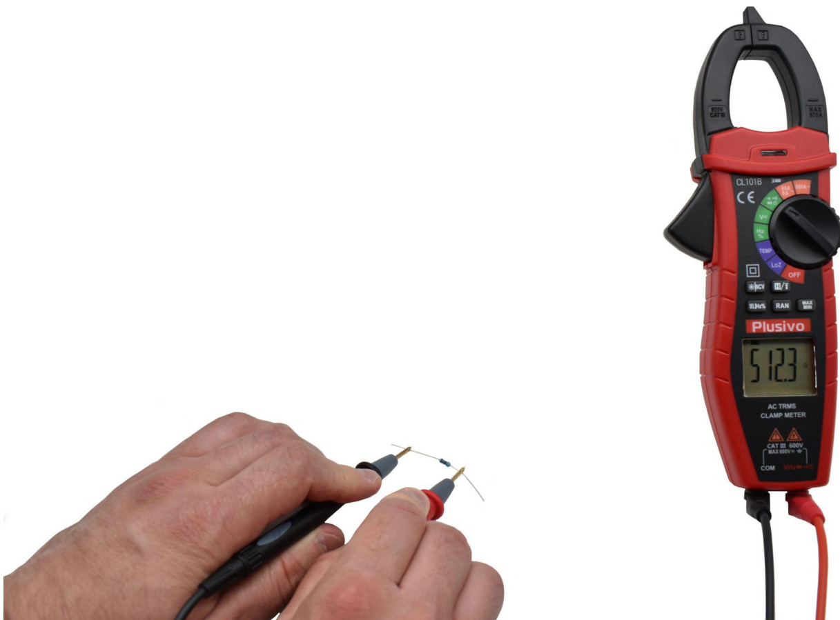
Figure 30. The measured resistance in this figure is 512.3 \Omega
