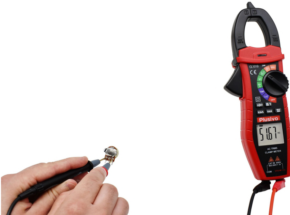
Figure 42. The measured resistance in this figure is 51.67 kΩ
