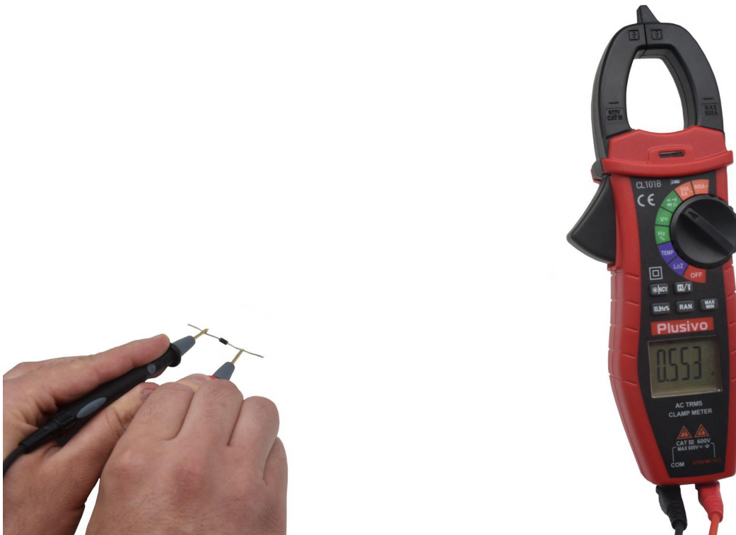
Figure 10. The measured forward voltage in this figure is 0.553 V
