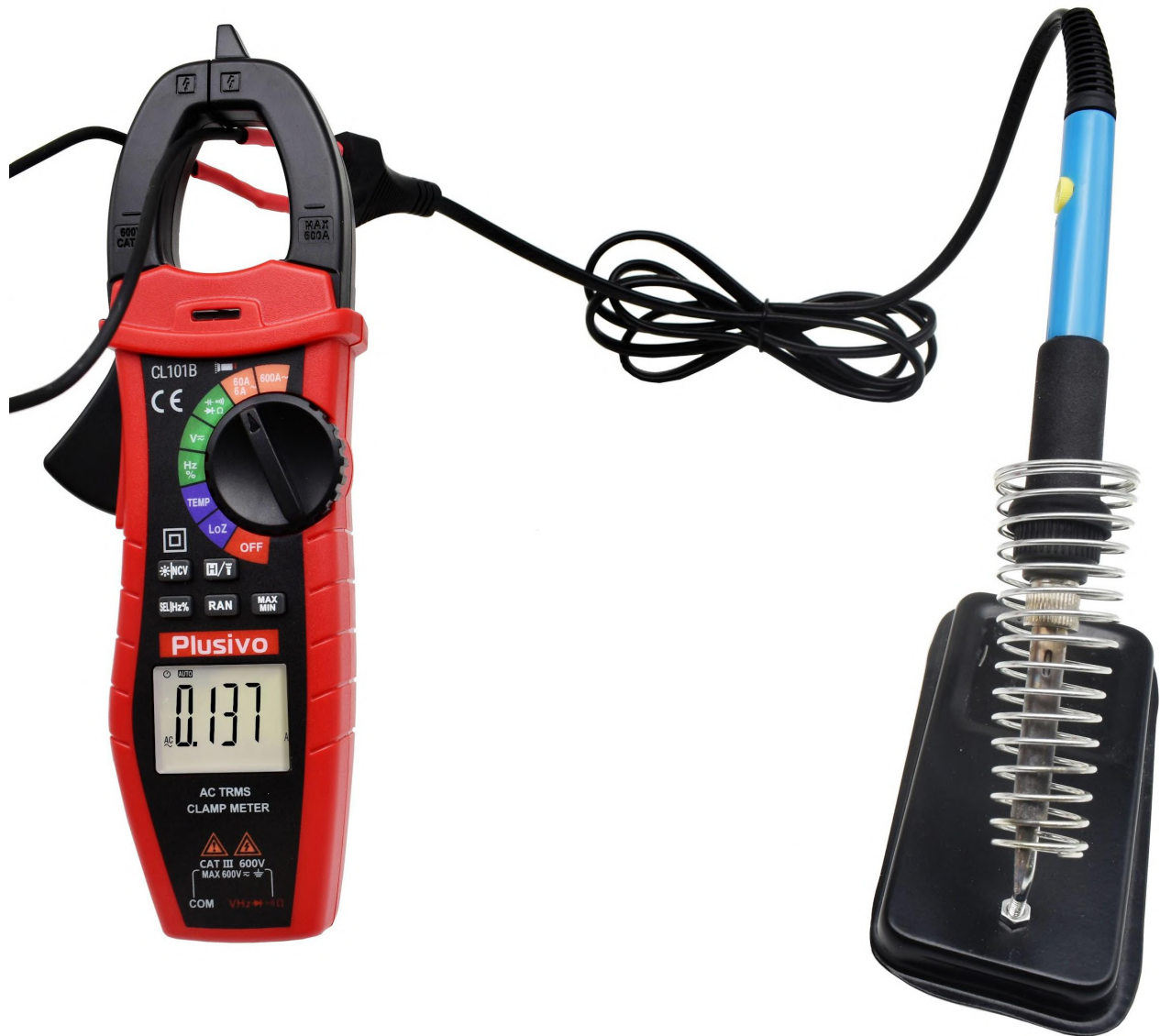
Figure 3. The measured current in this figure is 0.137 A AC
