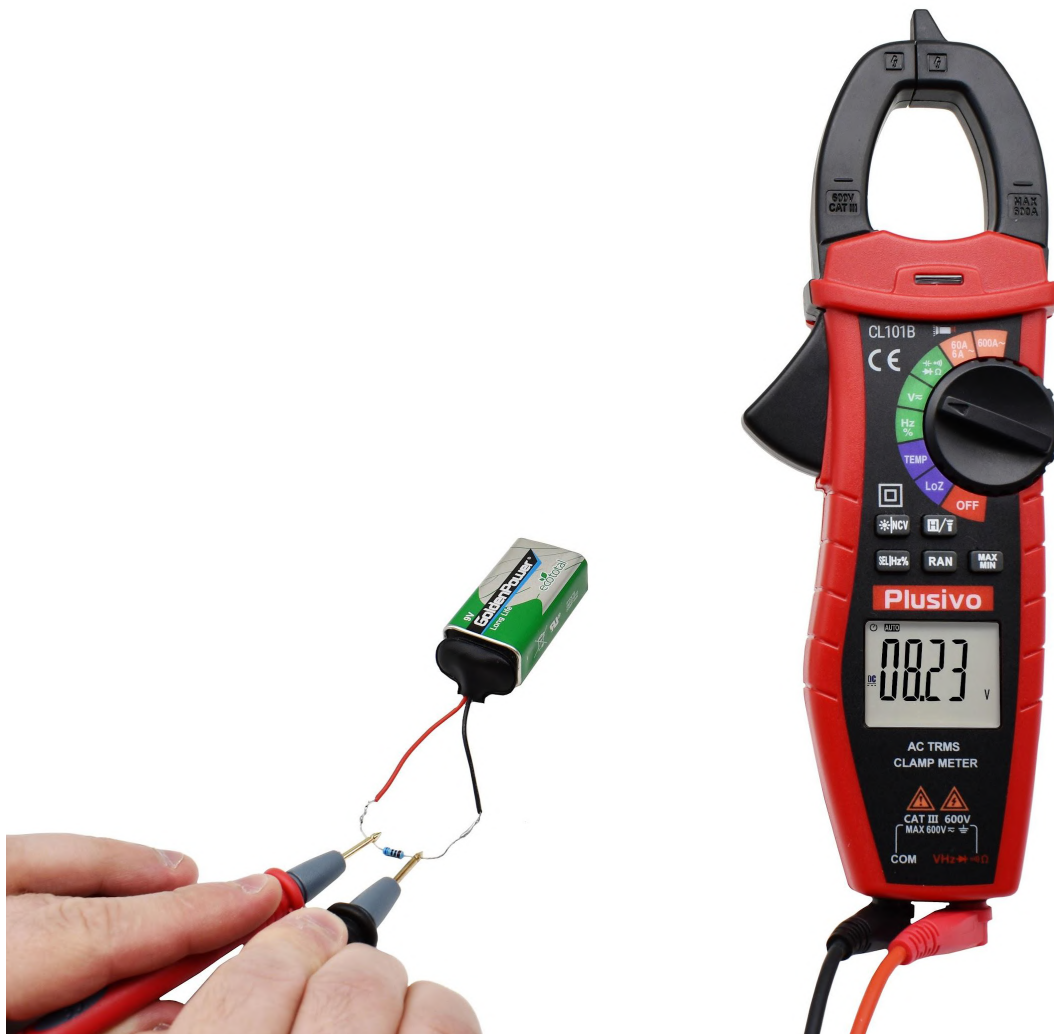
Figure 41. The measured voltage in this figure is 8.23 V DC
