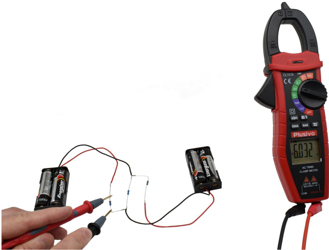
Figure 34. The measured voltage in this figure is 6.032 V DC
