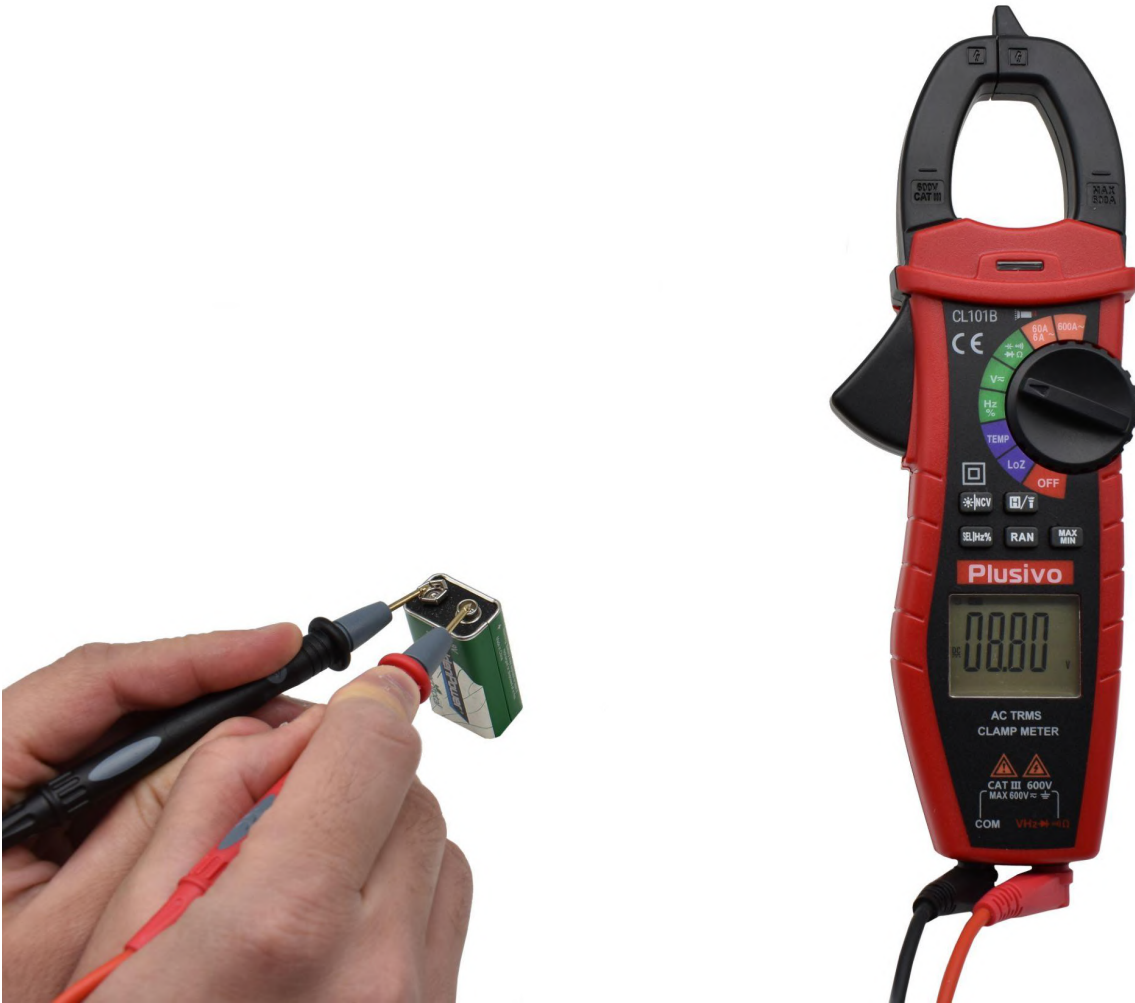
Figure 40. The measured voltage in this figure is 8.80 V DC
