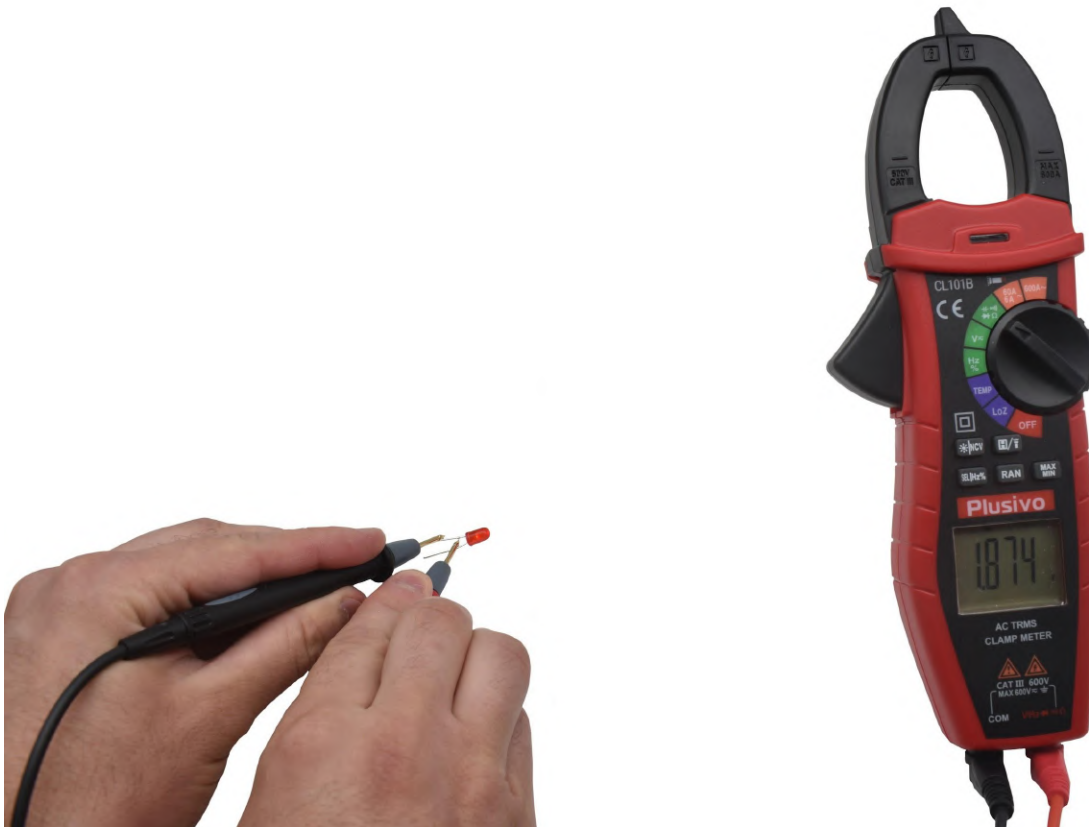
Figure 39. The measured forward voltage in this figure is 1.874 V
