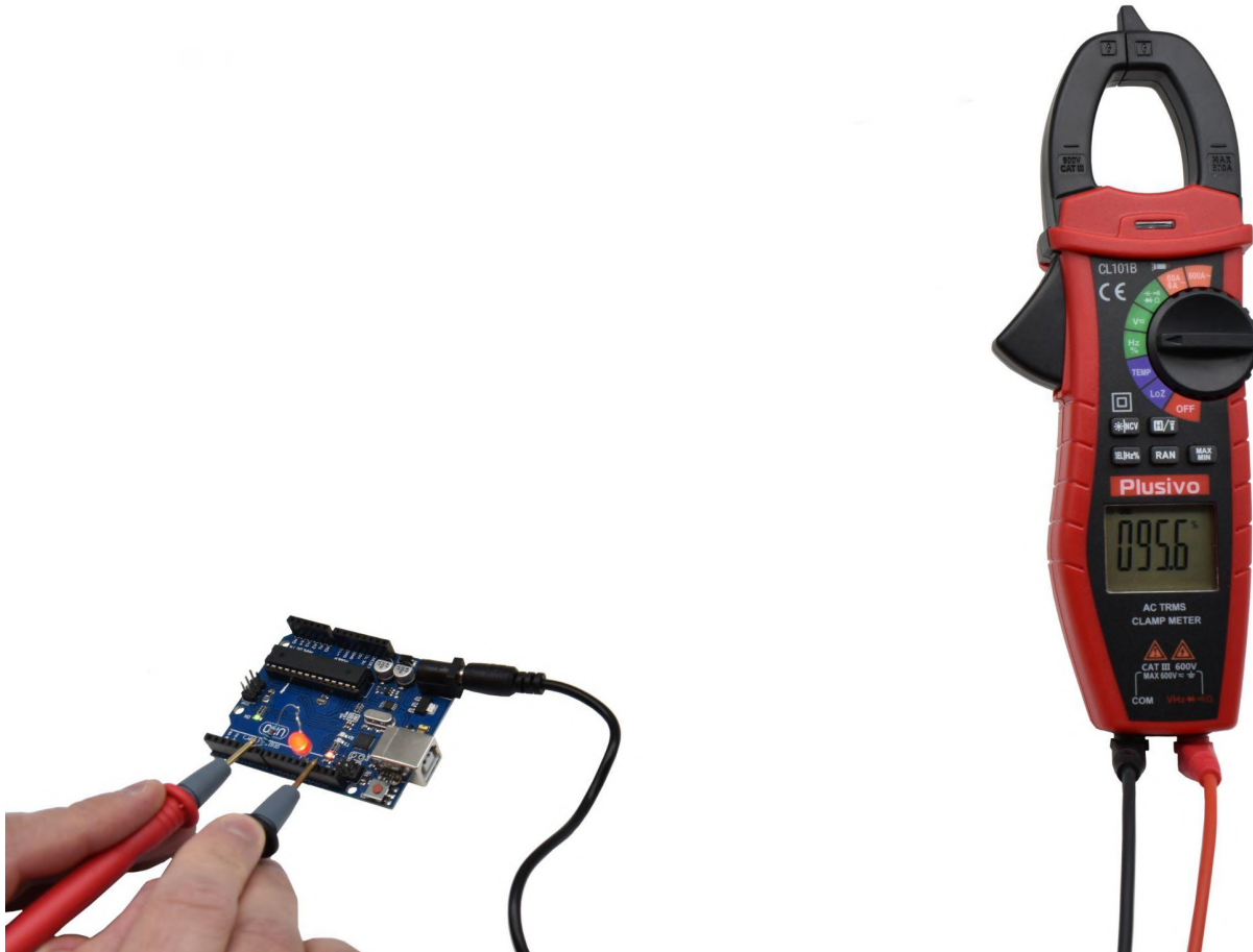
Figure 19. The measured duty cycle in this figure is 95.6 %
