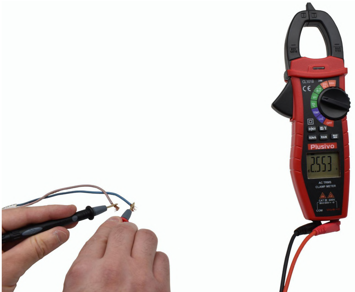
Figure 27. The measured voltage in this figure is 2.553 V AC
