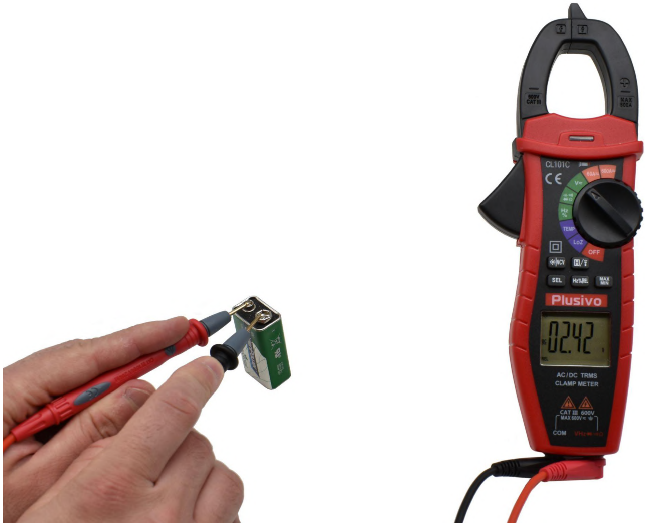
Figure 26. The measured voltage in this figure is 2.42 V DC
