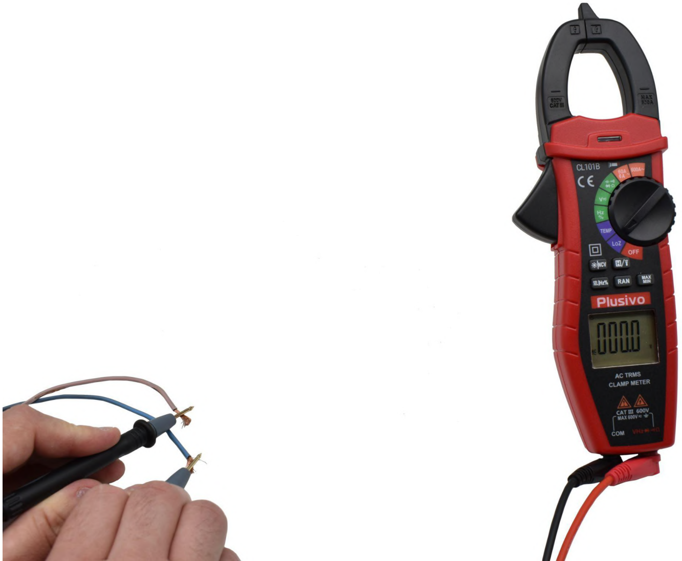
Figure 28. The measured voltage in this figure is 0.0 V AC
