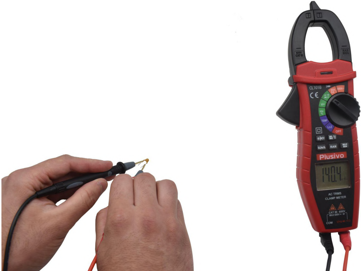
Figure 8. The measured capacitance in this figure is 140.4 nF
